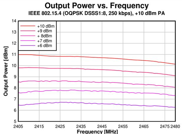
Figure 8-32. Output Power vs. Frequency (250 kbps, +10 dBm PA)
