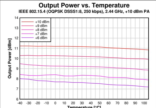
Figure 8-24. Output Power vs. Temperature (2.44 GHz, +10 dBm PA)
