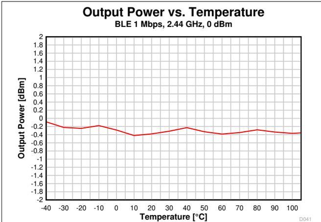
Figure 8-21. Output Power vs. Temperature (BLE 1 Mbps, 2.44 GHz)
