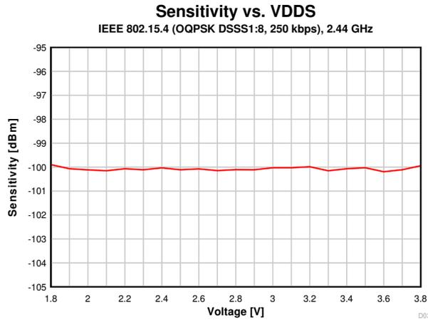
**Figure 8-20. Sensitivity vs. Supply Voltage (VDDS) (250 kbps, 2.44 GHz)**
