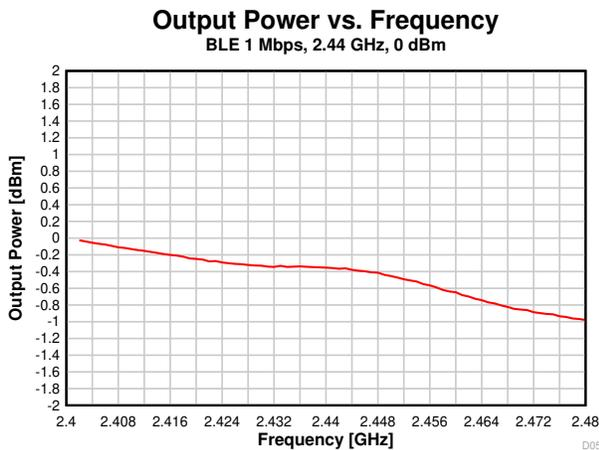
Figure 8-29. Output Power vs. Frequency (BLE 1 Mbps, 2.44 GHz)
