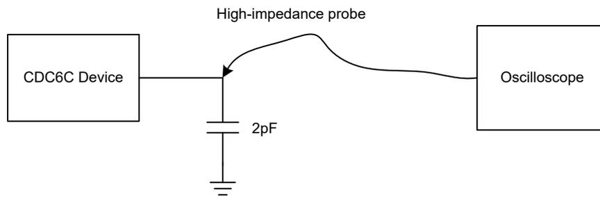
Load capacitor modified based on measurement condition.
