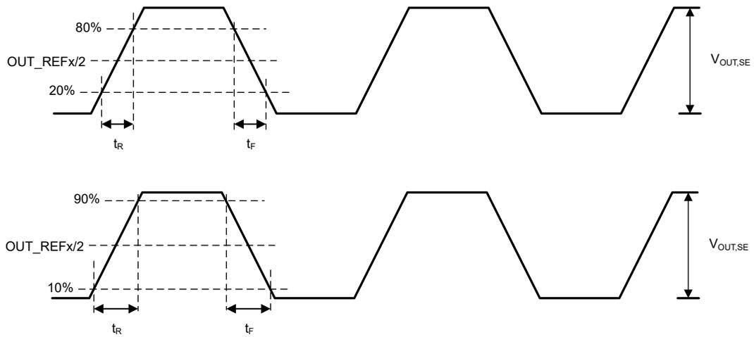
**Figure 6-1. Single-Ended Output Voltage and Rise/Fall Time**
