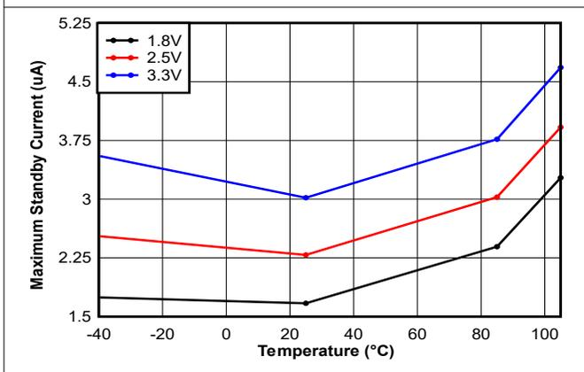
**Figure 6-7. Maximum Standby Current vs Temperature and Supply Voltage**
