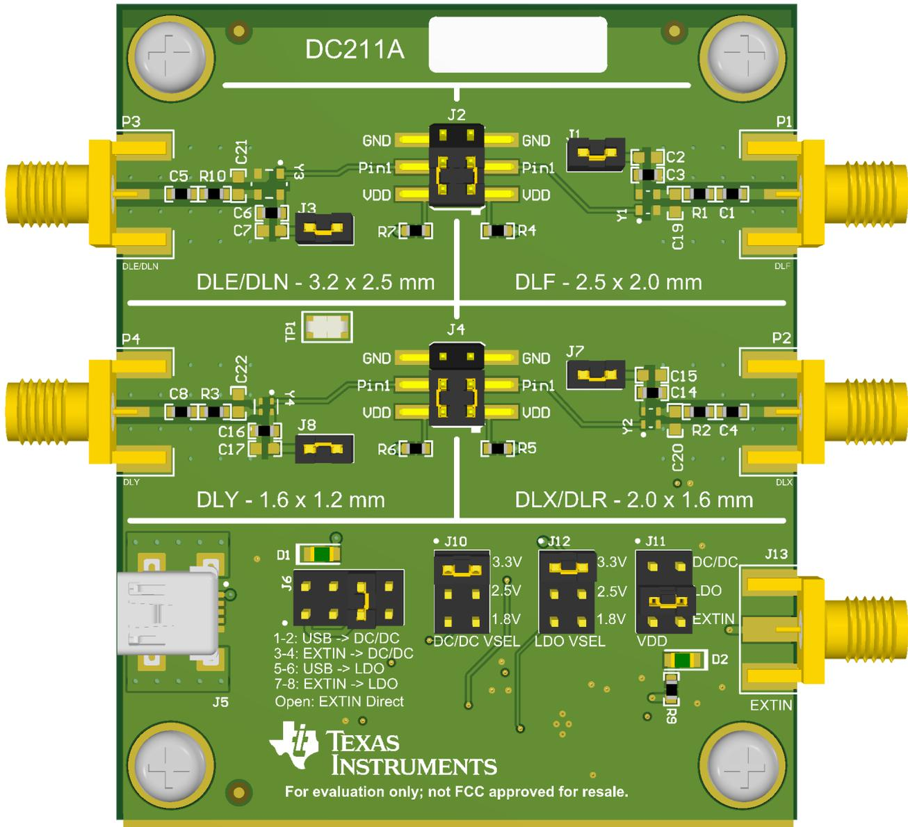
Figure 9-10. PCB Layout Example From CDC6 EVM
