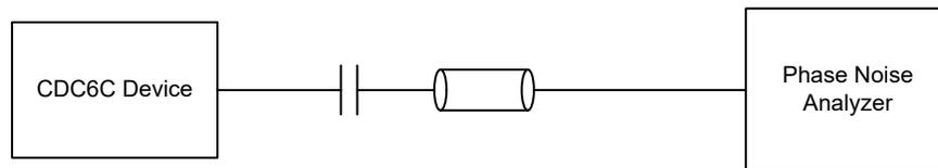
**Figure 7-2. CDC6Cx Output Phase Noise Test Configuration**
