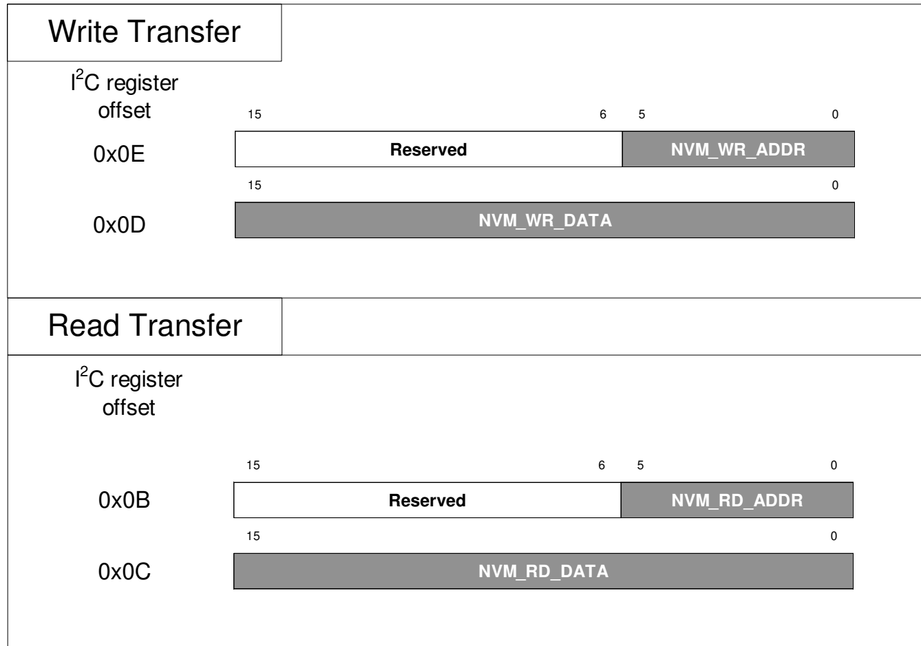
Figure 10-11. EEPROM Direct Access Using I 2 C
