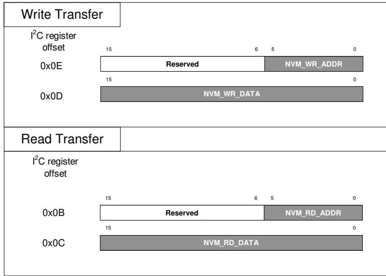
Figure 8-12. EEPROM Direct Access Using I 2 C
