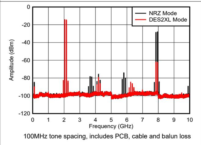
**Figure 6-46. Dual Tone,  $f_{\text{OUT}} = 2097\text{MHz}$ , 0dBFS**
