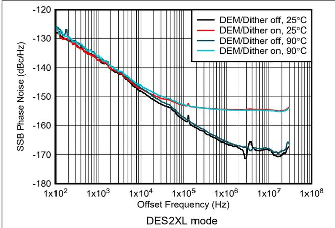
**Figure 6-220. Phase Noise vs Offset Frequency at 1GHz**
