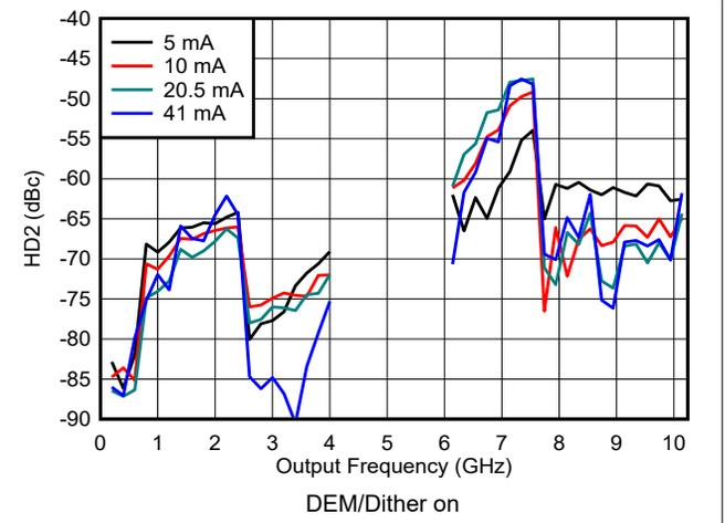
**Figure 6-159. HD2 vs Frequency and Output Current in DES2X Modes**
