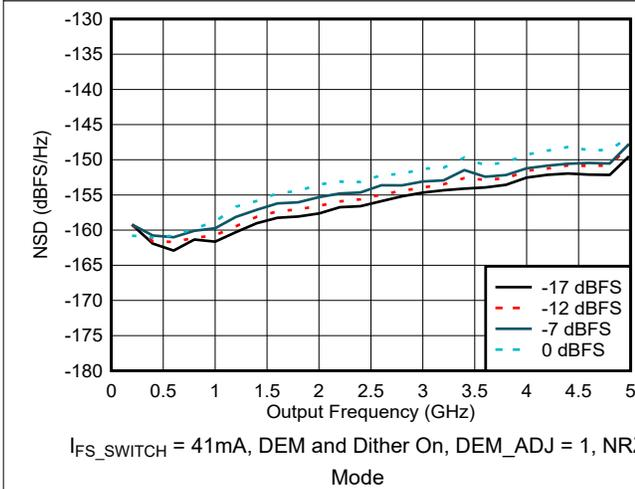
Figure 6-70. NSD vs Output Frequency and Digital Amplitude
