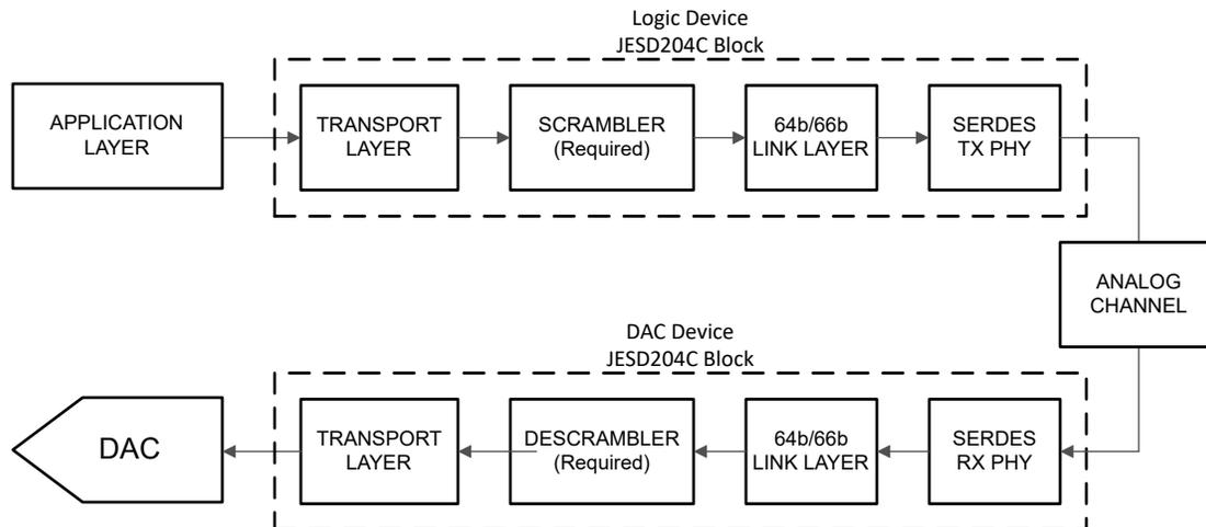
Figure 7-51. Simplified JESD204C Interface Diagram with 64b/66b Encoding
