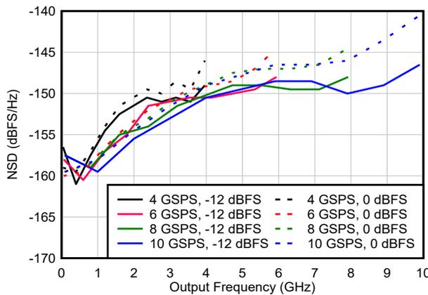
$I_{FS\_SWITCH} = 20.5\text{mA}$ , DEM and Dither On, NRZ and RF
