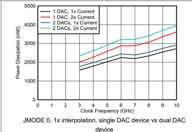
**Figure 6-93. Power Dissipation vs Clock Frequency and DAC Mode**
