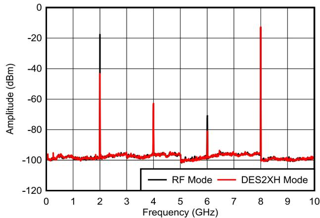
**Figure 9-4. Output Spectra Comparing DES2XH and RF Modes**
