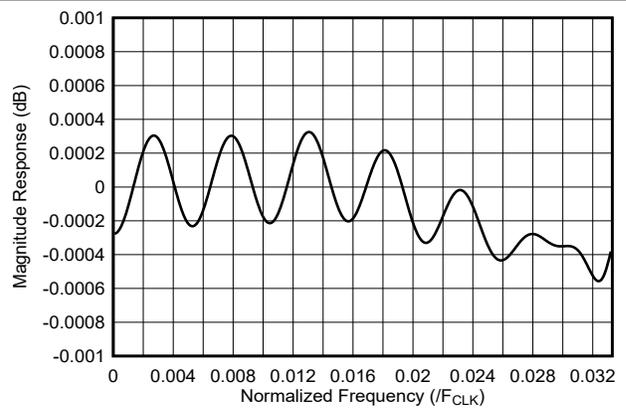
**Figure 7-25. 12x Interpolation Filter Passband Response**
