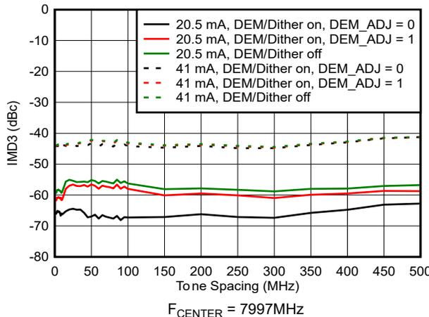
**Figure 6-142. IMD3 vs Tone Spacing in RF Mode**
