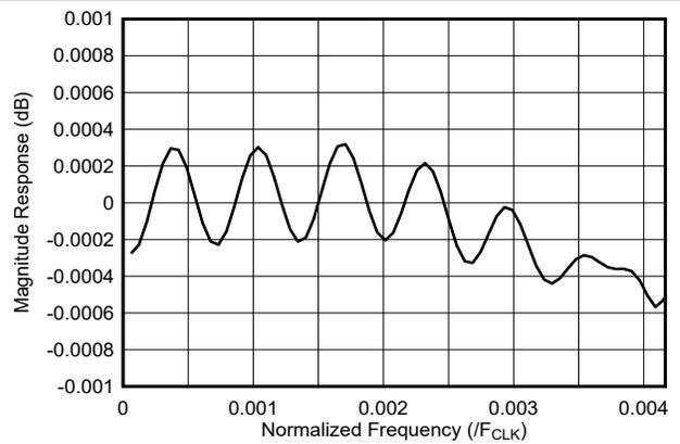
**Figure 7-37. 96x Interpolation Filter Passband Response**
