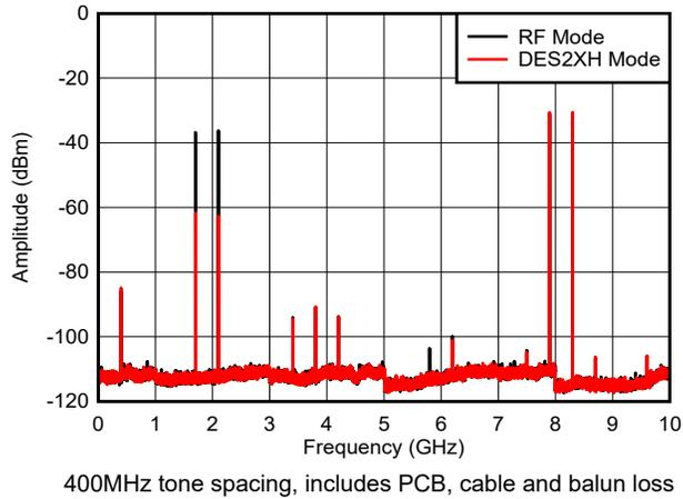
**Figure 6-57. Dual Tone,  $f_{\text{OUT}} = 7997\text{MHz}$ ,  $-12\text{dBFS}$**
