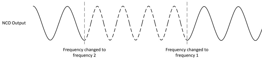
**Figure 7-44. Example Phase Continuous NCO Mode Operation**
