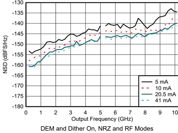
Figure 6-62. NSD vs Output Frequency and Output Current
