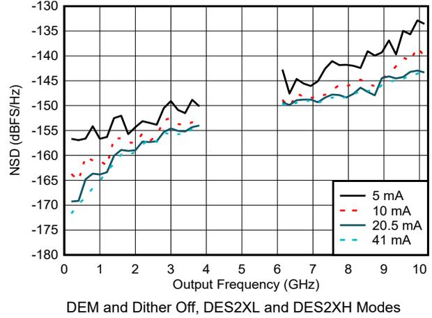
Figure 6-63. NSD vs Output Frequency and Output Current
