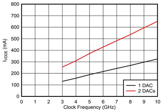
Independent of JMODE, Interpolation, single DAC device vs dual DAC device
