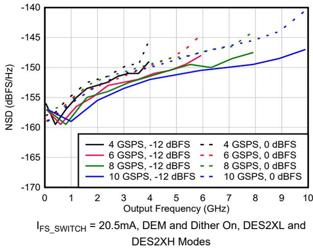
**Figure 6-80. NSD vs Output Frequency and Sample Rate**
