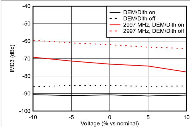
Figure 6-152. IMD3 vs Voltage in NRZ Mode
