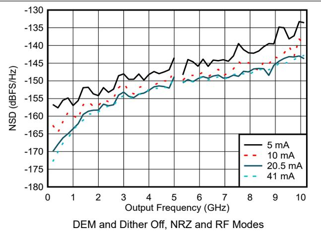
Figure 6-61. NSD vs Output Frequency and Output Current
