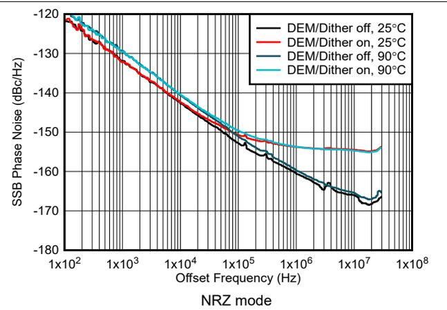
Figure 6-219. Phase Noise vs Offset Frequency at 1GHz
