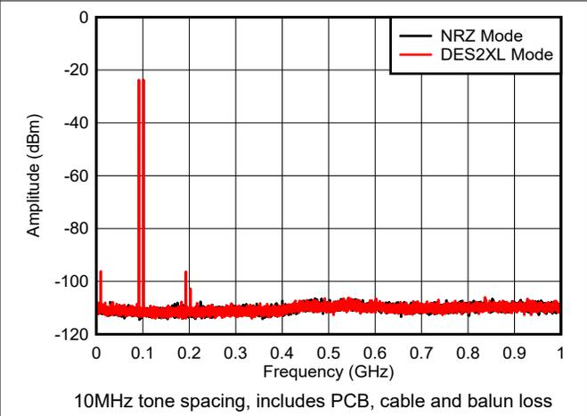
**Figure 6-42. Dual Tone,  $f_{\text{OUT}} = 97\text{MHz}$ , -6dBFS (0 - 1GHz)**
