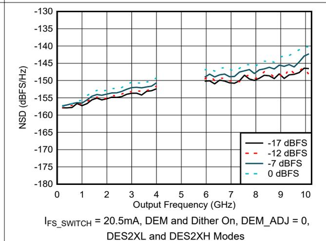
Figure 6-73. NSD vs Output Frequency and Digital Amplitude
