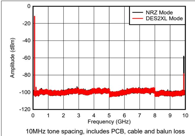
Figure 6-37. Dual Tone,  $f_{\text{OUT}} = 97\text{ MHz}$ , 0dBFS (0 -  $f_{\text{CLK}}$ )
