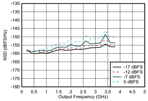
$I_{FS\_SWITCH} = 20.5\text{mA}$ , DEM and Dither On, DEM\_ADJ = 1,
