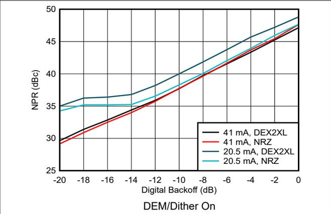
**Figure 6-211. Noise Power Ratio vs Digital Backoff: 1<sup>st</sup> Nyquist Zone**
