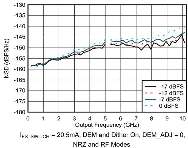
Figure 6-67. NSD vs Output Frequency and Digital Amplitude
