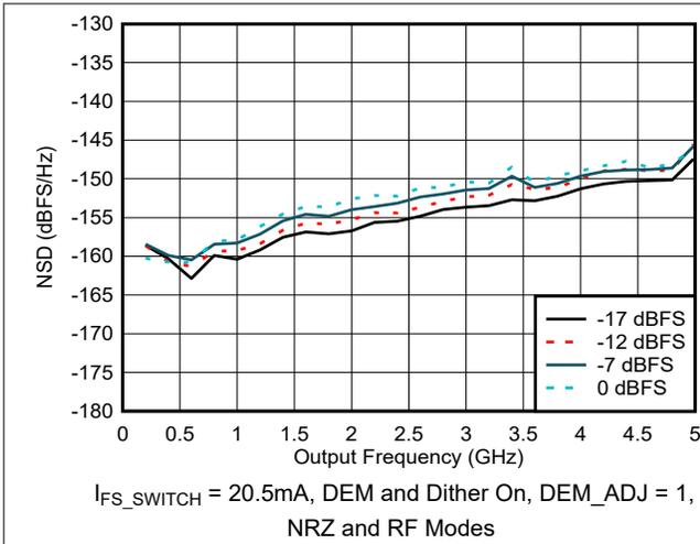
Figure 6-68. NSD vs Output Frequency and Digital Amplitude
