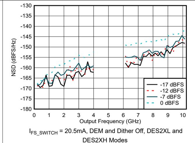
Figure 6-71. NSD vs Output Frequency and Digital Amplitude
