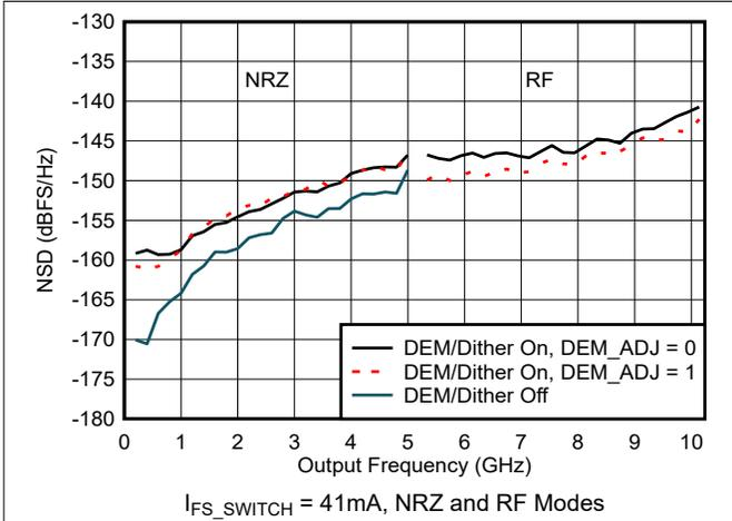
Figure 6-58. NSD vs Output Frequency and DEM/Dither Mode
