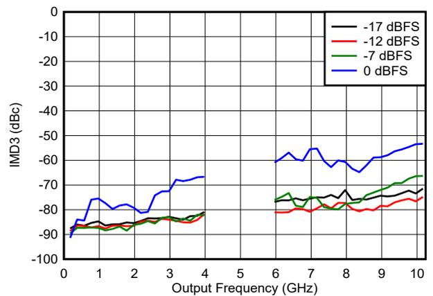
**Figure 6-137. IMD3 vs Frequency and Digital Amplitude in DES2X Modes**
