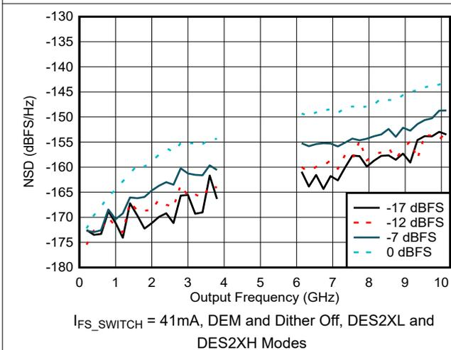
Figure 6-72. NSD vs Output Frequency and Digital Amplitude
