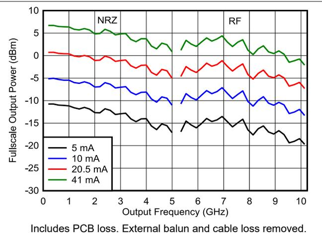
**Figure 6-9. Output Power vs Frequency (NRZ/RF modes)**
