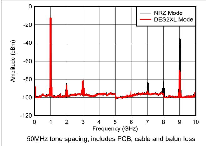
**Figure 6-43. Dual Tone,  $f_{\text{OUT}} = 997\text{MHz}$ , 0dBFS**
