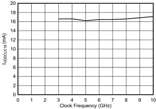
Independent of JMODE, interpolation, and single/dual DAC device
