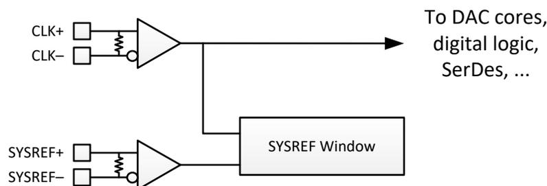
**Figure 7-12. Device Clocking Subsystem**
