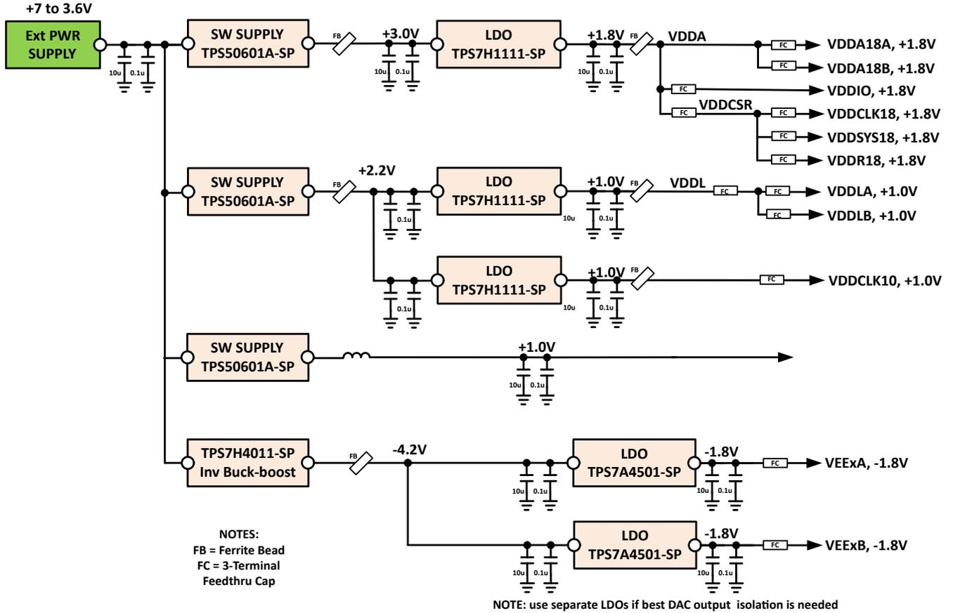
Figure 9-20. Recommended -SP Power Supply Block Diagram
