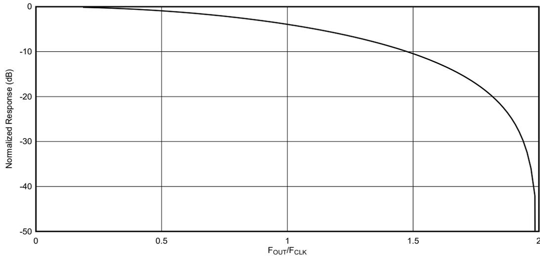
**Figure 7-10. DES1X Output Frequency Response**
