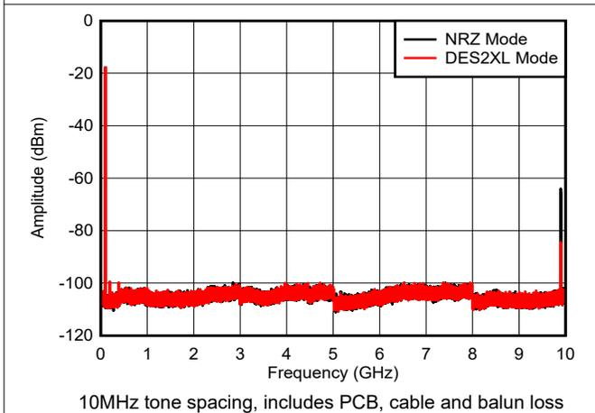
Figure 6-39. Dual Tone,  $f_{\text{OUT}} = 97\text{ MHz}$ , -6dBFS (0 -  $f_{\text{CLK}}$ )
