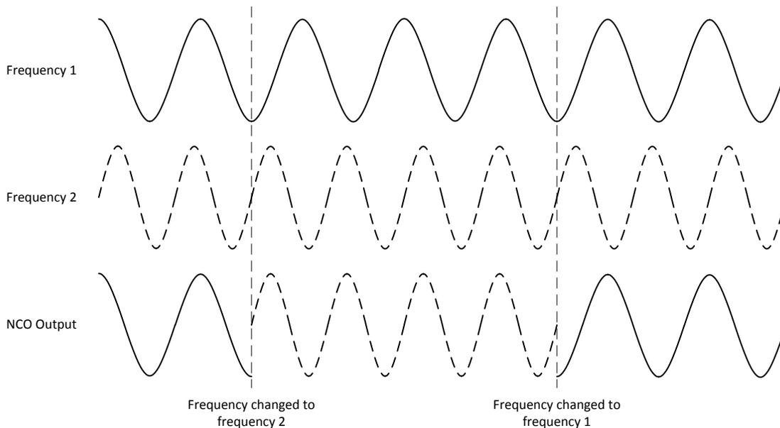
**Figure 7-45. Example Phase Coherent NCO Mode Operation**
