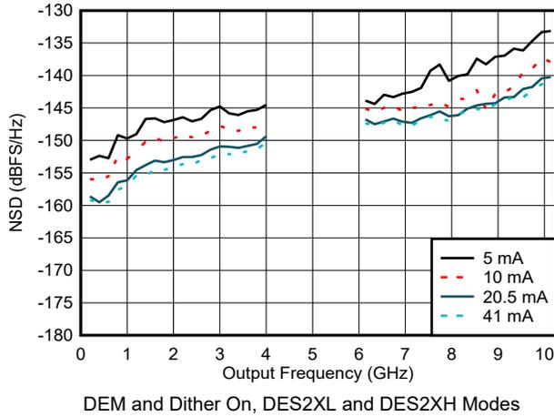
Figure 6-64. NSD vs Output Frequency and Output Current
