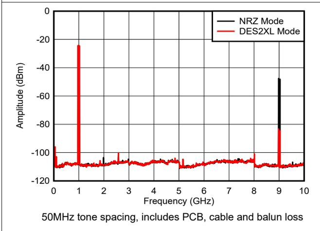
**Figure 6-45. Dual Tone,  $f_{\text{OUT}} = 997\text{MHz}$ , -12dBFS**
