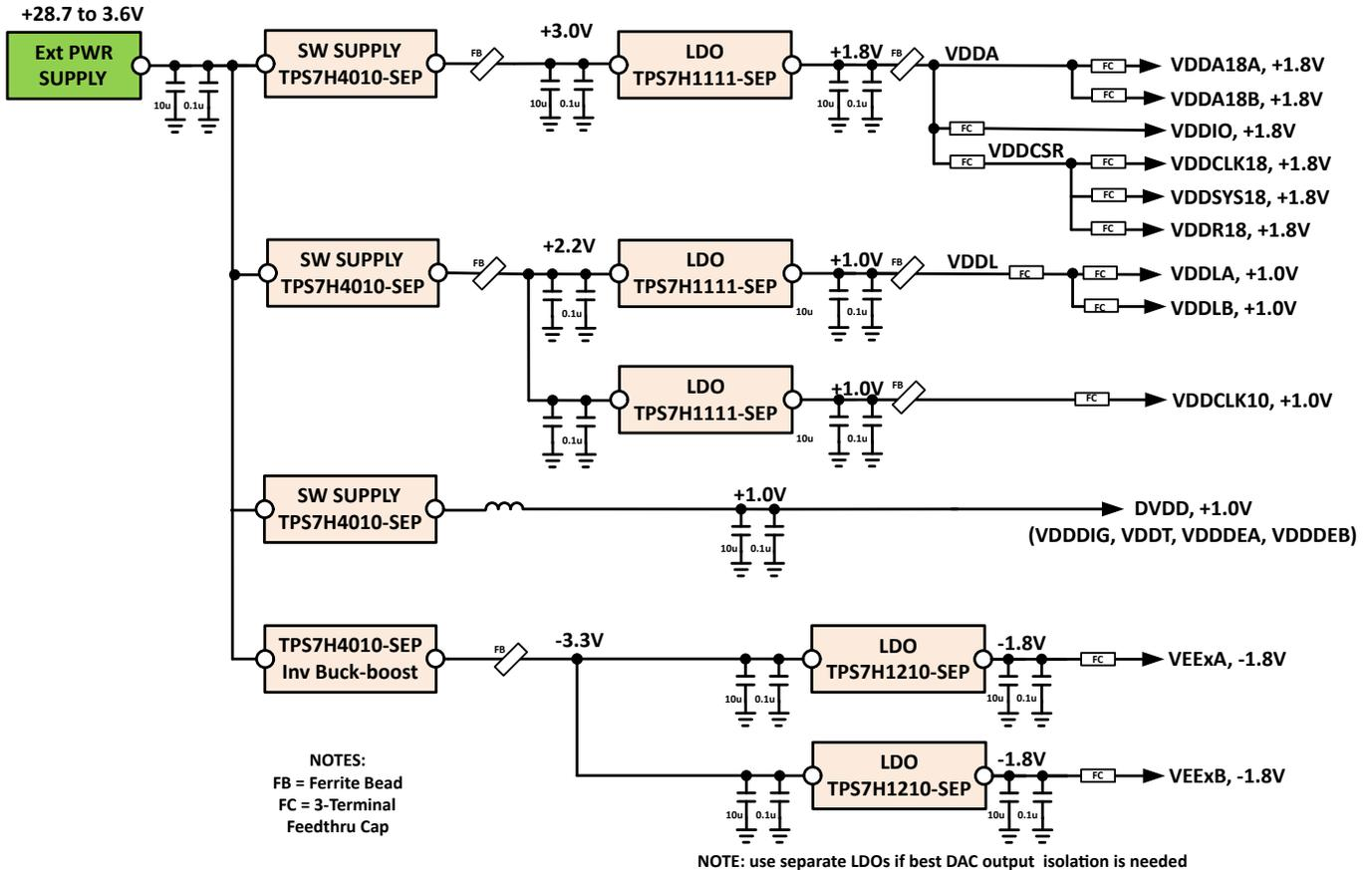
Figure 9-21. Recommended -SEP Power Supply Block Diagram
