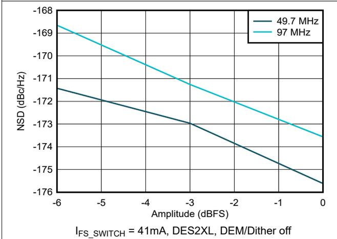
Figure 6-60. NSD vs Digital Amplitude at Low Frequency
