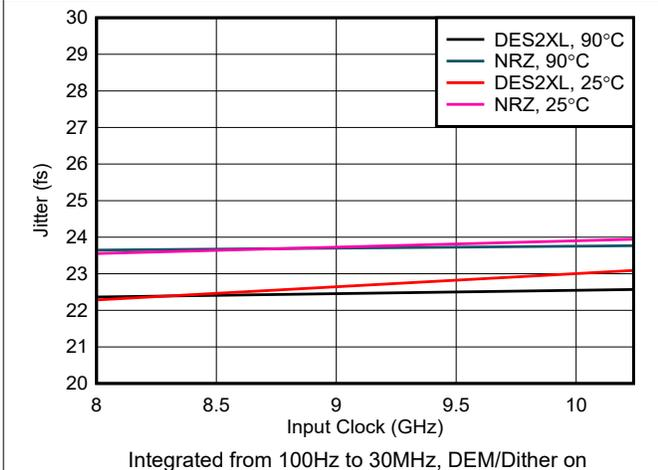
**Figure 6-222. Jitter vs Input Clock**
