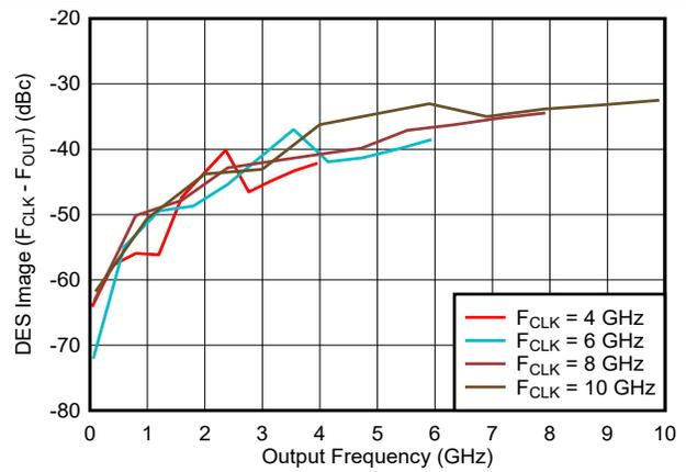
DES Image =  $F_{CLK} - F_{OUT}$ . DES Image relative to power of the tone at the same frequency as the image using the inverse DES2X mode. This removes the bandwidth difference across frequency.
