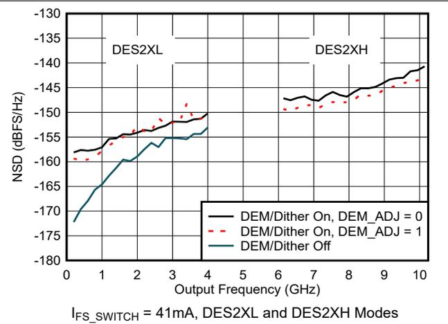
Figure 6-59. NSD vs Output Frequency and DEM/Dither Mode
