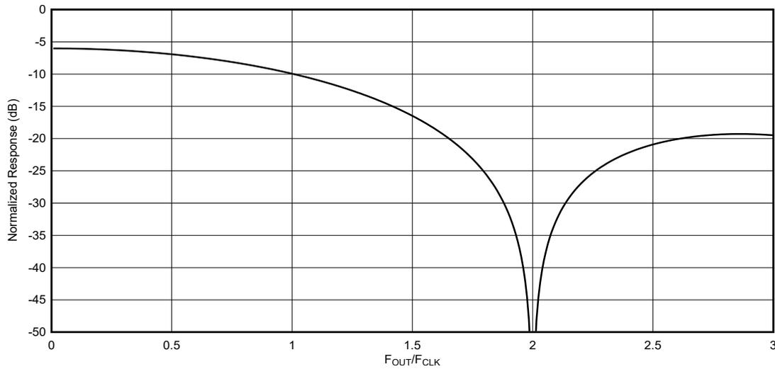
**Figure 7-6. RTZ Mode Output Frequency Response**
