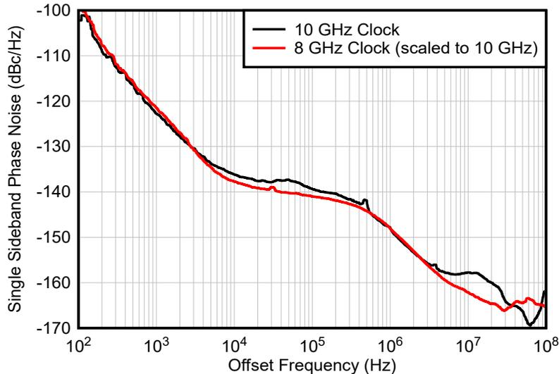
**Figure 9-12. 8GHz and 10GHz Clock Phase Noise**
