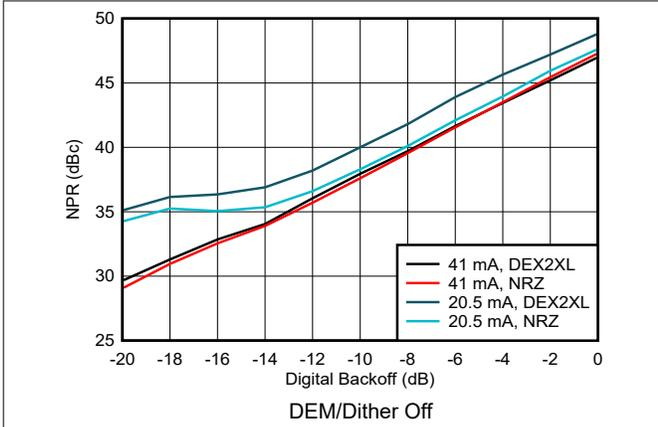
**Figure 6-210. Noise Power Ratio vs Digital Backoff: 1<sup>st</sup> Nyquist Zone**
