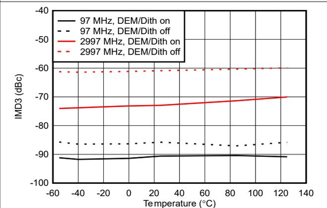
**Figure 6-149. IMD3 vs Temperature in DES2XL Mode**
