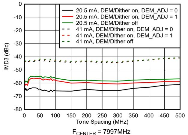
**Figure 6-143. IMD3 vs Tone Spacing in DES2XH Mode**
