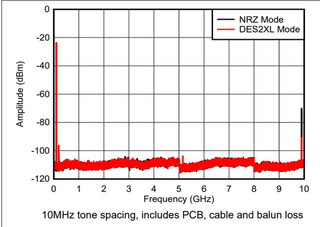
**Figure 6-41. Dual Tone,  $f_{\text{OUT}} = 97\text{MHz}$ , -12dBFS (0 -  $f_{\text{CLK}}$ )**
