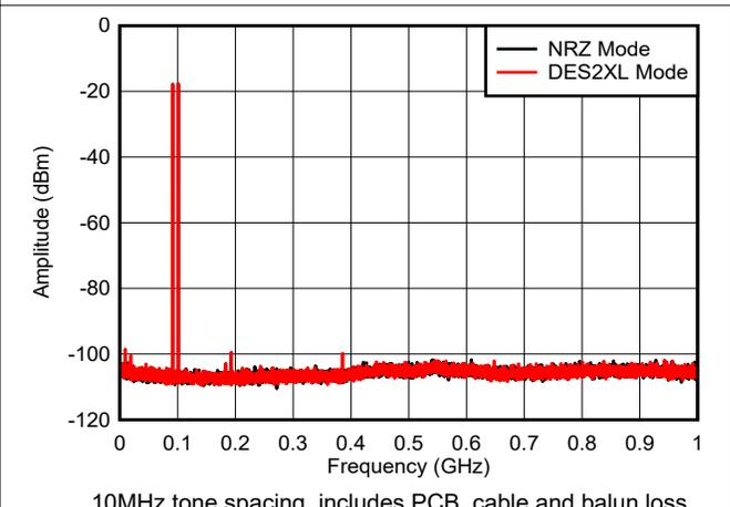
Figure 6-40. Dual Tone,  $f_{\text{OUT}} = 97\text{ MHz}$ , -6dBFS (0 - 1GHz)
