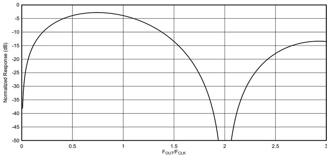
Figure 7-8. RF Mode Output Frequency Response
