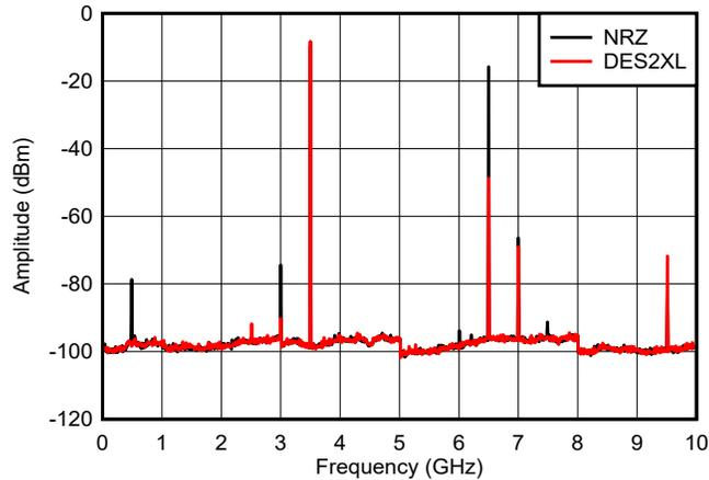
**Figure 9-3. Output Spectra Comparing DES2XL and NRZ Modes**
