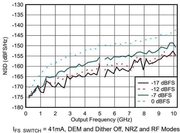
Figure 6-66. NSD vs Output Frequency and Digital Amplitude
