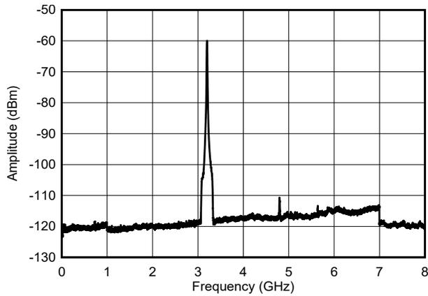
**Figure 9-17. NLFM Chirp Output Spectra Across 0 - 8GHz**
