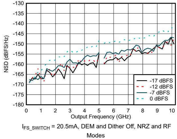
Figure 6-65. NSD vs Output Frequency and Digital Amplitude
