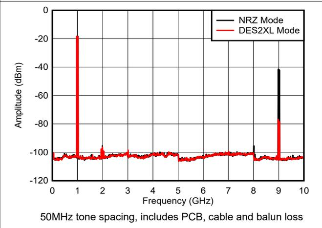
**Figure 6-44. Dual Tone,  $f_{\text{OUT}} = 997\text{MHz}$ , -6dBFS**
