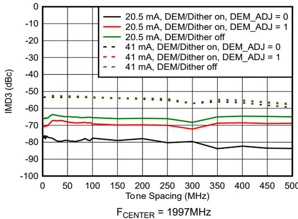
**Figure 6-140. IMD3 vs Tone Spacing in NRZ Mode**
