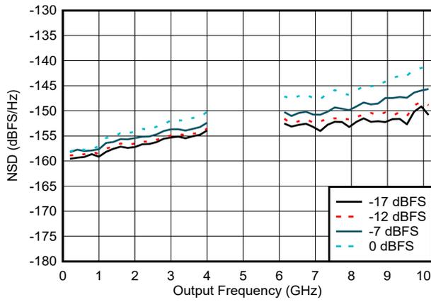
$I_{FS\_SWITCH} = 41\text{mA}$ , DEM and Dither On, DEM\_ADJ = 0,
