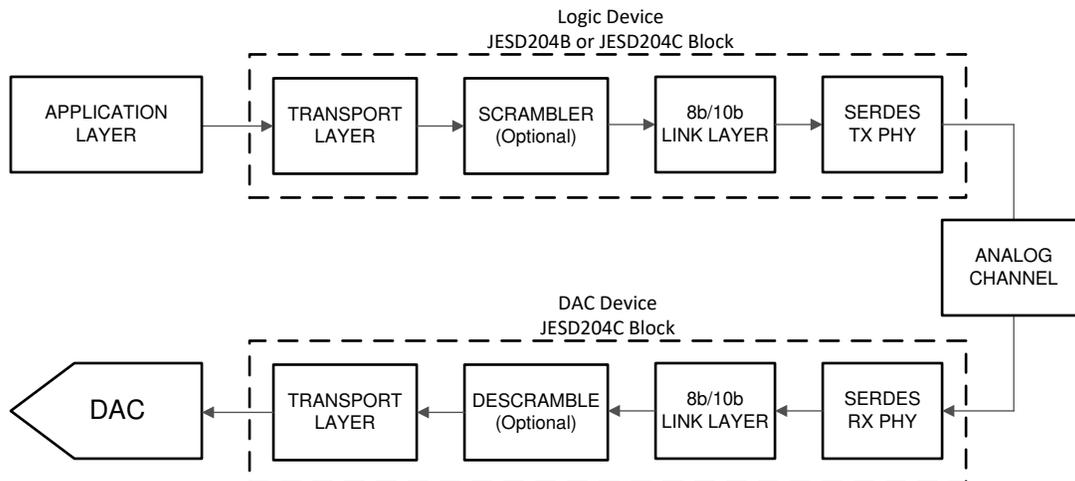
**Figure 7-50. Simplified JESD204C Interface Diagram with 8b/10b Encoding**
