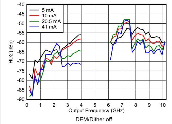
**Figure 6-158. HD2 vs Frequency and Output Current in DES2X Modes**
