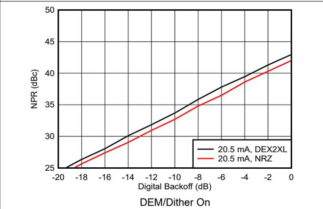
**Figure 6-213. Noise Power Ratio vs Digital Backoff: 2<sup>nd</sup> Nyquist Zone**
