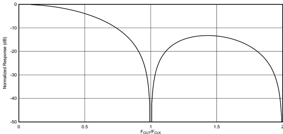
**Figure 7-4. NRZ Mode Output Frequency Response**
