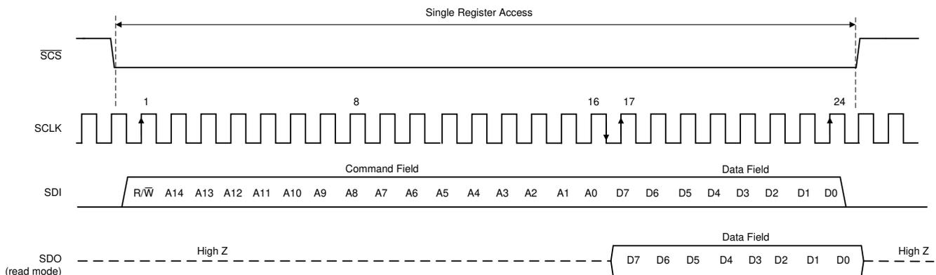
**Figure 7-58. Serial Interface Protocol: Single Read and Write**
