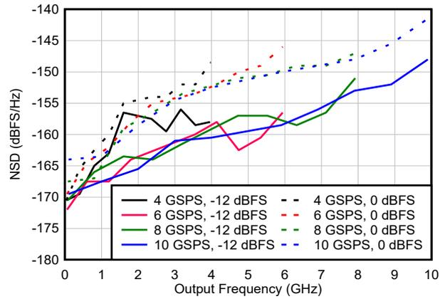
$I_{FS\_SWITCH} = 20.5\text{mA}$ , DEM and Dither Off, NRZ and RF
