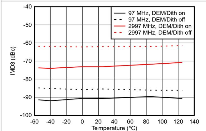
**Figure 6-148. IMD3 vs Temperature in NRZ Mode**
