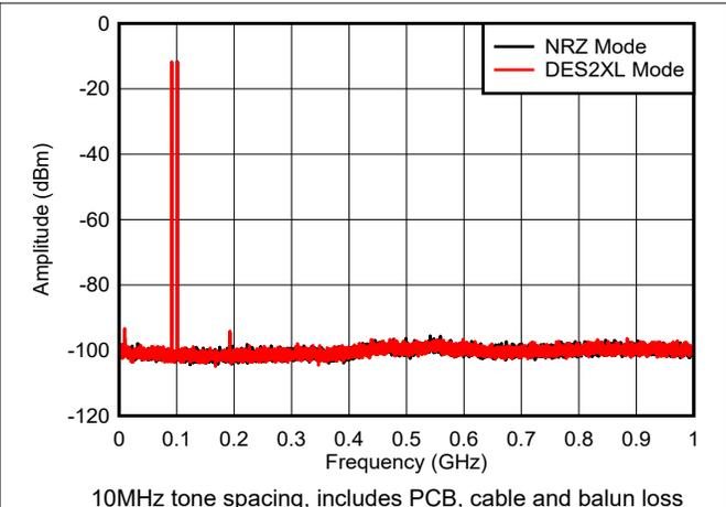
Figure 6-38. Dual Tone,  $f_{\text{OUT}} = 97\text{ MHz}$ , 0dBFS (0 - 1GHz)
