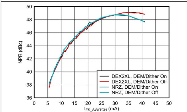
**Figure 6-214. Noise Power Ratio vs Output Current: 1<sup>st</sup> Nyquist Zone**
