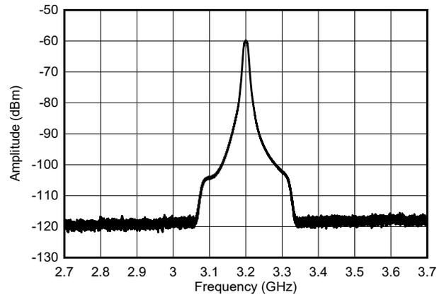
**Figure 9-18. NLFM Chirp Output Spectra Across 1GHz**
