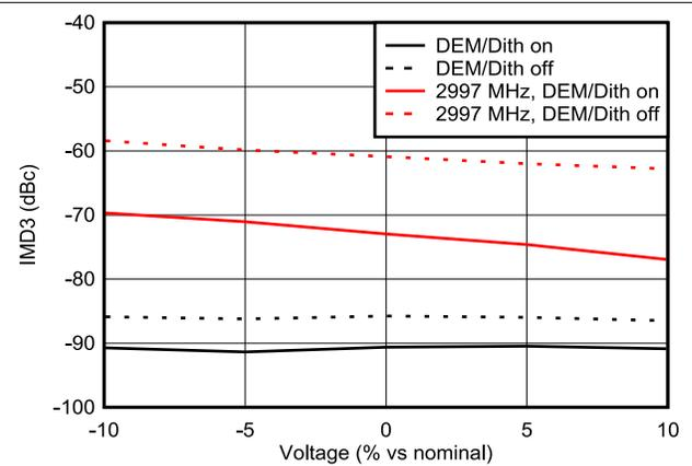
Figure 6-153. IMD3 vs Voltage in DES2XL Mode
