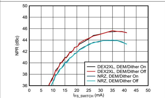
**Figure 6-215. Noise Power Ratio vs Output Current: 2<sup>nd</sup> Nyquist Zone**
