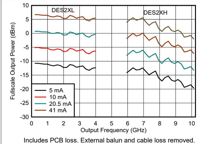
**Figure 6-10. Output Power vs Frequency (DES2X modes)**
