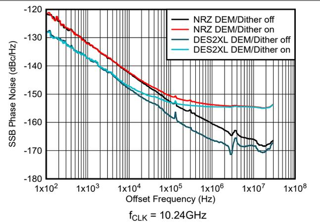
Figure 6-217. Phase Noise vs Offset Frequency at 1GHz
