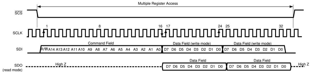
**Figure 7-59. Serial Interface Protocol: Streaming Read and Write**
