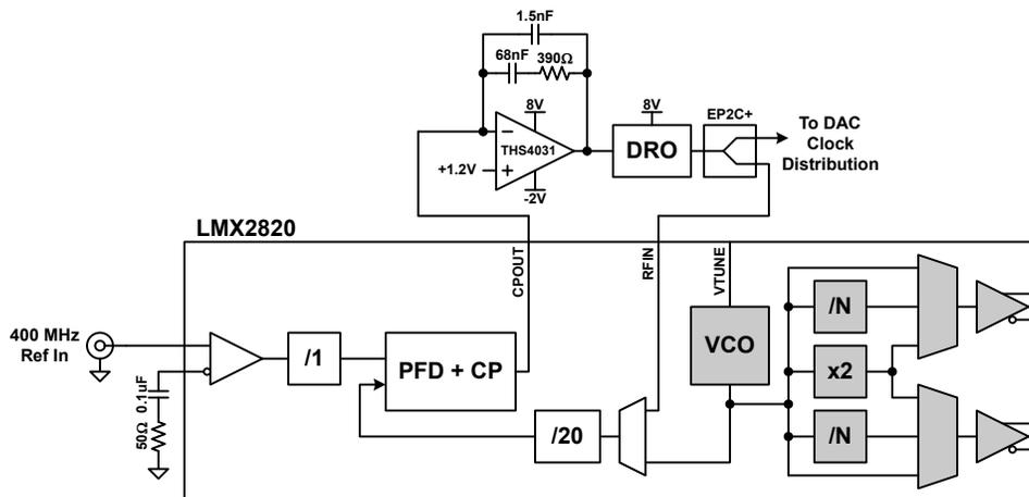
**Figure 9-8. External LMX2820 with an External VCO**
