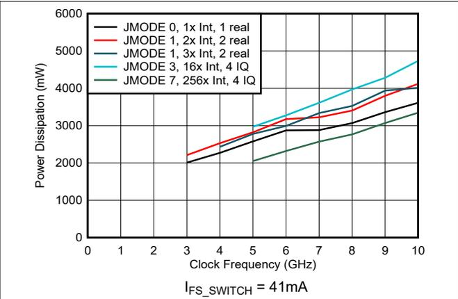
**Figure 6-90. Power Dissipation vs Clock Frequency and Digital Mode**
