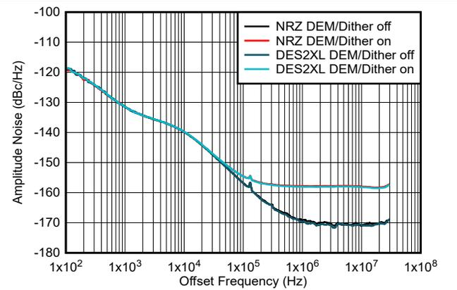
**Figure 6-223. Amplitude Noise vs Offset Frequency at 1GHz**
