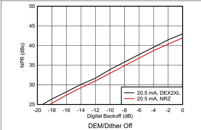
**Figure 6-212. Noise Power Ratio vs Digital Backoff: 2<sup>nd</sup> Nyquist Zone**
