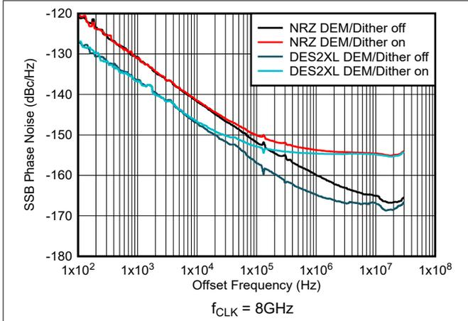
Figure 6-216. Phase Noise vs Offset Frequency at 1GHz
