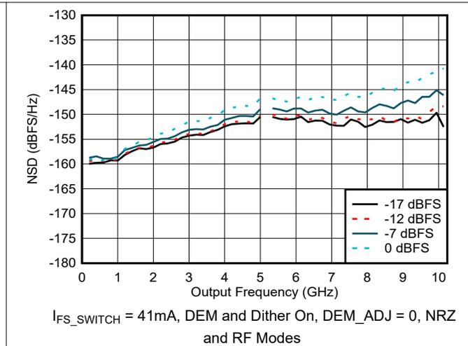
Figure 6-69. NSD vs Output Frequency and Digital Amplitude
