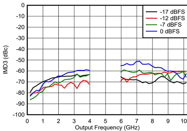
**Figure 6-136. IMD3 vs Frequency and Digital Amplitude in DES2X Modes**
