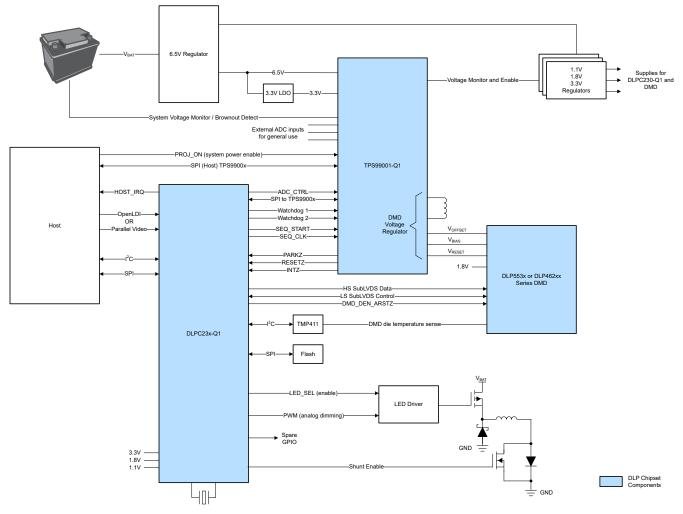
Figure 8-2 shows the system block diagram for a DLP<sup>®</sup> headlight.
