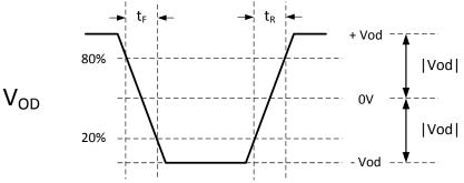
Differential Output Signal (Note:  $V_{CM}$  is removed when signals are viewed differentially)
