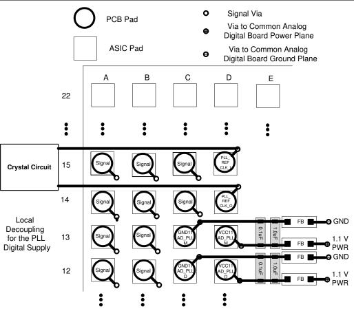
Figure 8-11. DLPC230-Q1 PLL Filter Layout
