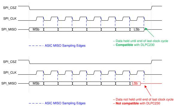
Figure 5-10. TPS99000-Q1 Interface Data Capture Requirements
