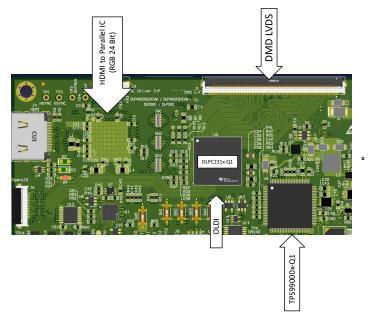
Figure 8-16. Top level Layout Example—OLDI and DMD LVDS
