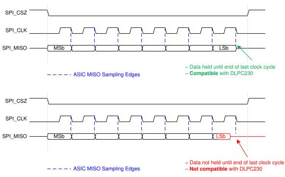
Figure 5-8. Flash Interface Data Capture Requirements
