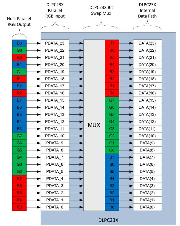
Figure 7-2. Example of Alternate Parallel Port Bit Mapping
