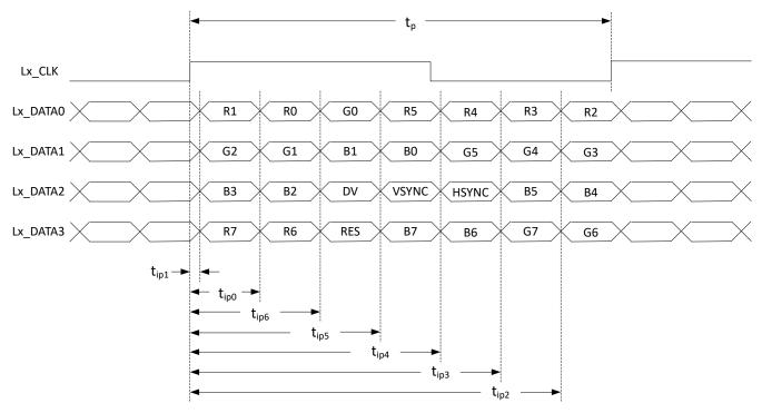
Figure 5-4. OpenLDI Interface Timing
