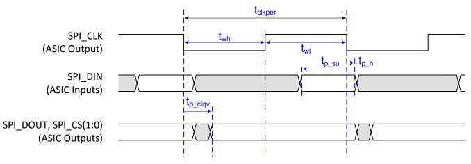
Figure 5-7. Flash Interface Timing
