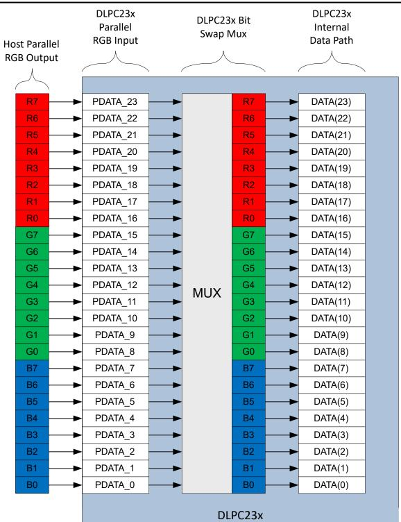
Figure 7-1. Example of Typical Parallel Port Bit Mapping
