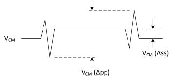
(2) Note that V<sub>OD</sub> is the differential voltage swing measured across a 100Ω termination resistance connected directly between the transmitter differential pins. |V<sub>OD</sub>| is the magnitude of the peak to peak voltage swing across the P and N output pins. Because V<sub>CM</sub> cancels out when measured differentially, V<sub>OD</sub> voltage swings relative to 0. Rise and fall times are defined for the differential V<sub>OD</sub> signal as follows:
