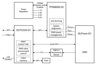
DLP553x-Q1 or DLP4621-Q1 DLP<sup>®</sup> Chipset System Block Diagram
