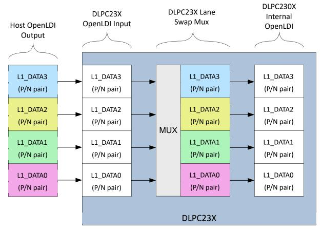
Figure 7-3. Example of Typical OpenLDI Port Lane Mapping
