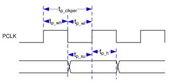
Figure 5-3. Parallel Interface General Timing
