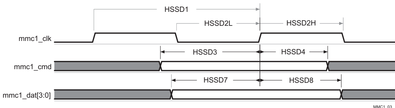
Figure 5-85. MMC/SD/SDIO in - High Speed - Receiver Mode
