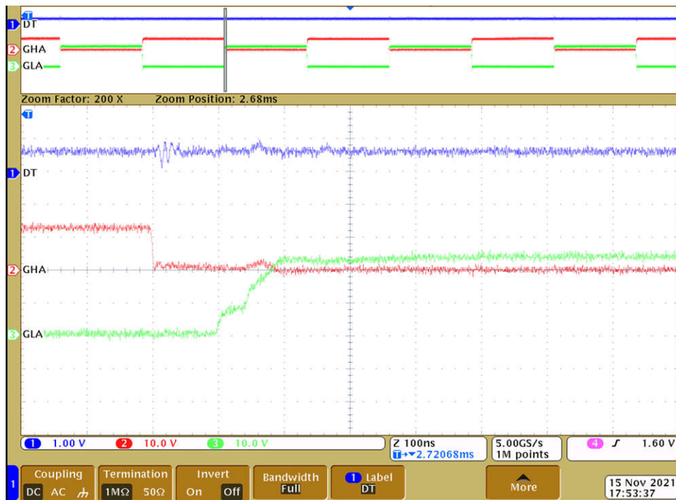
Figure 8-16. Driver dead time of 100 ns (DT = 10 kΩ to GND)
