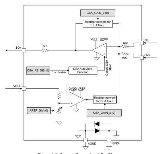
Figure 6-9. Current-Sense Amplifier Diagram
