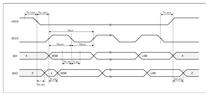
Figure 5-1. SPI Slave Mode Timing Diagram
