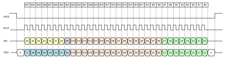
Figure 6-25. SPI Format - 32-bit frame (SPI\_CRC\_EN = 1b)
