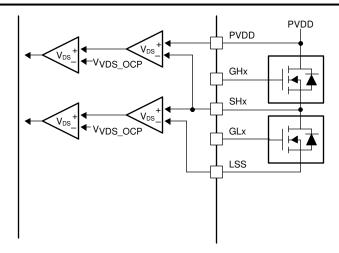
Figure 6-19. DRV8334-Q1 V<sub>DS</sub> Monitors
