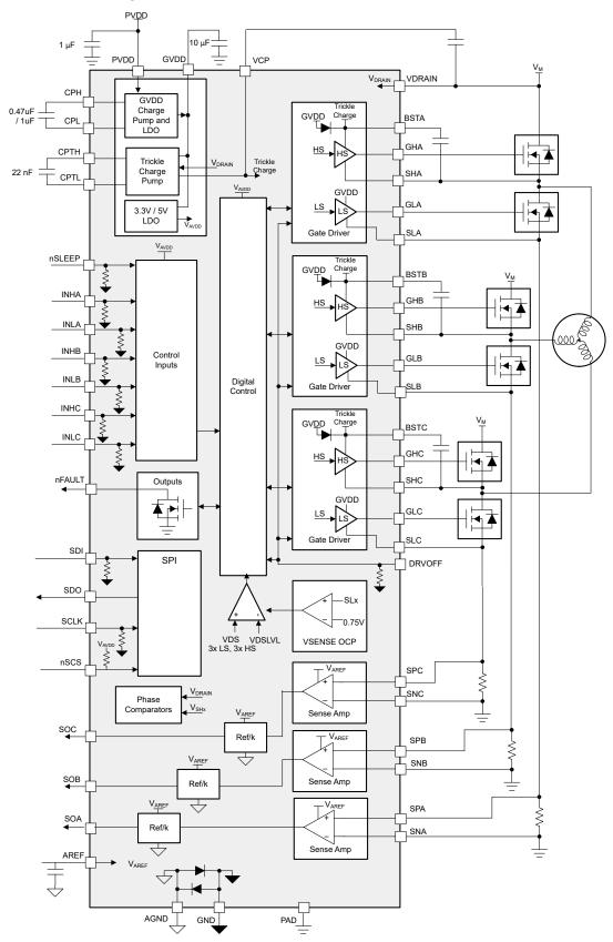
Figure 6-1. Block Diagram of DRV8334-Q1
