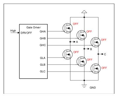
Figure 6-14. DRVOFF Gate Driver Output State
