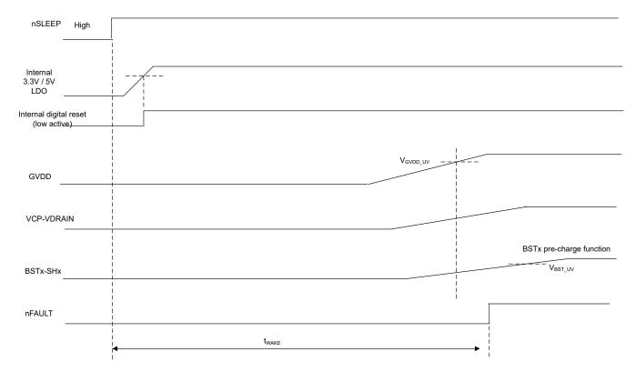
Figure 6-24. Device Power Up Sequence and twake
