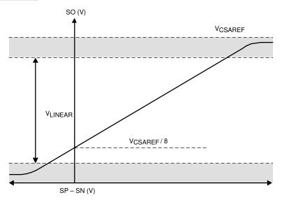
Figure 6-10. Unidirectional Current-Sense Output
