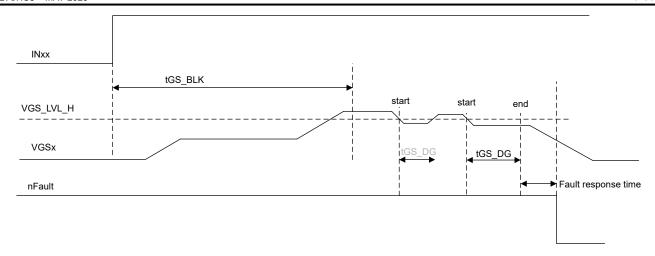
Figure 6-17. DRV8334-Q1 V<sub>GS</sub> Monitor Timing (Output High)
