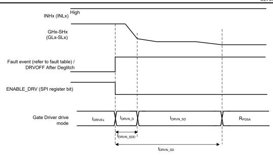
Figure 6-15. Gate Drive Shutdown Sequence
