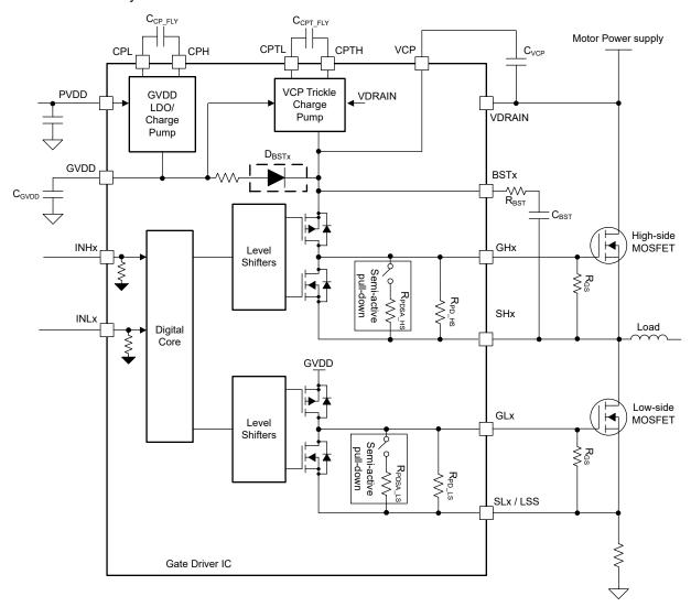
Figure 6-5. Gate Driver Architecture
