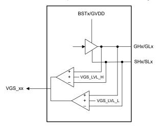
Figure 6-16. DRV8334-Q1 V<sub>GS</sub> Monitors
