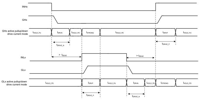
Figure 6-6. TDRIVE Gate Drive Timing Control (DEADT\_MODE = 0b)
