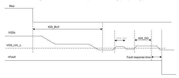
Figure 6-18. DRV8334-Q1 V<sub>GS</sub> Monitor Timing (Output Low)
