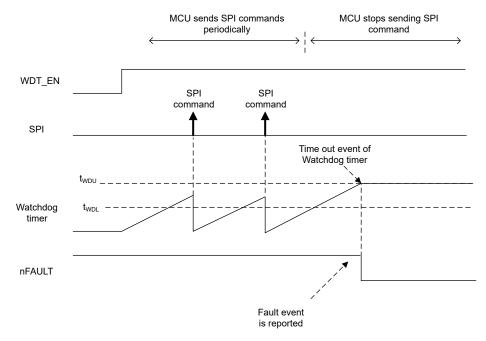
Figure 6-22. SPI Watchdog Timer timing diagram
