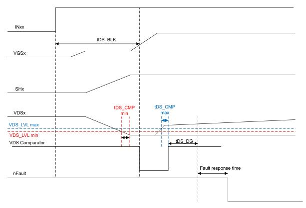
Figure 6-20. DRV8334-Q1 V<sub>DS</sub> Monitor Timing
