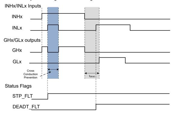
Figure 6-8. Cross Conduction Prevention and Dead time Insertion
