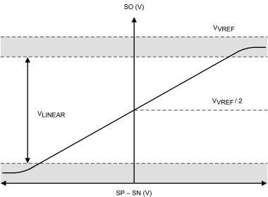
Figure 6-12. Bidirectional Current Sense Output
