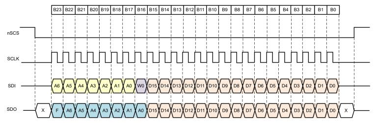
Figure 6-26. SPI Format - 24-bit frame (SPI\_CRC\_EN = 0b)
