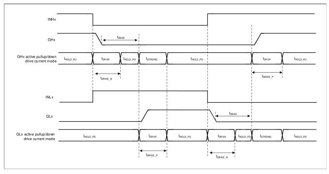
Figure 6-7. TDRIVE Gate Drive Timing Control (DEADT\_MODE = 1b)
