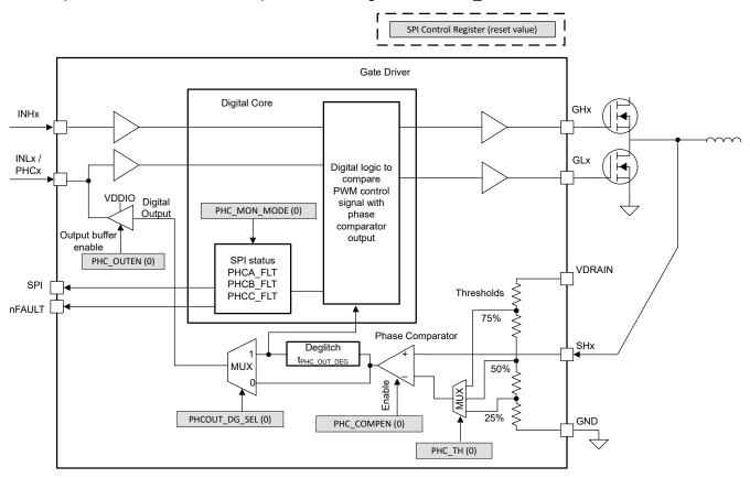
Figure 6-21. Phase Comparator Functional Diagram
