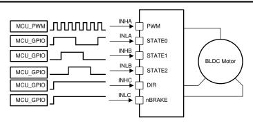
Figure 6-2. 1x PWM—Simple Controller
