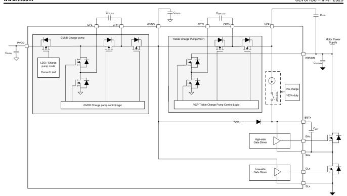
Figure 6-4. DRV8334-Q1 Gate Driver Power Supply Architecture
