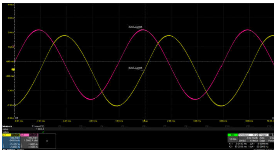
Figure 7-20. Coil Current Waveform with Silent Step Decay
