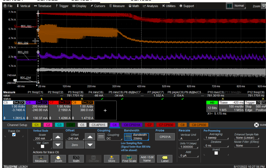
Figure 8-3. Driving four brushed-DC motors
