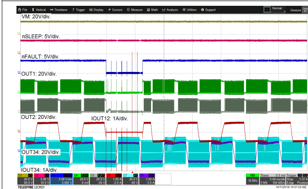
Figure 8-15. Over Current Protection and Recovery
