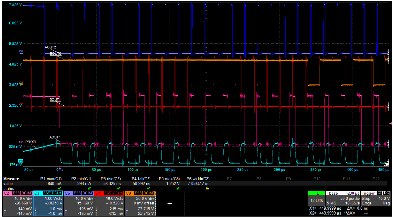
Figure 8-2. Driving four loads simultaneously
