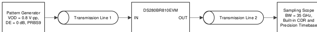
Figure 20. 10 in Rx and 5 in Tx Channel Test Setup
