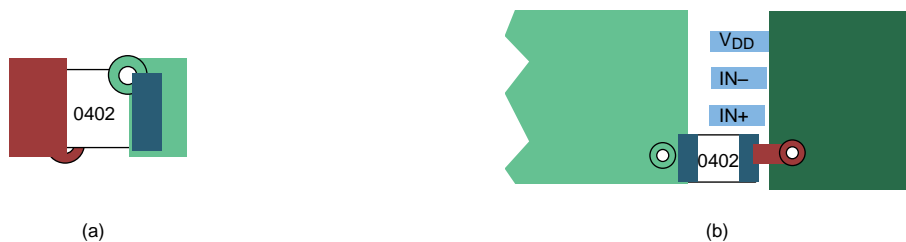
Figure 21. Typical Decoupling Capacitor Layouts
