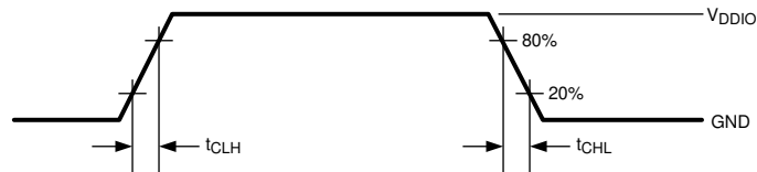
Figure 6-1. LVCMOS Transition Times
