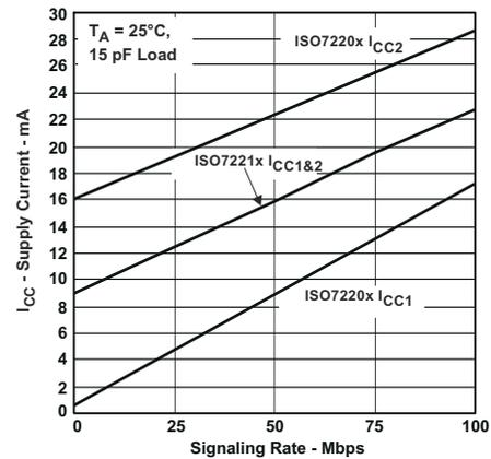
**Figure 5-3. 5-V<sub>RMS</sub> Supply Current vs Signaling Rate (Mbps)**
