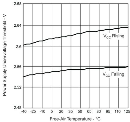
**Figure 5-10. V<sub>CC</sub> Undervoltage Threshold vs Free-Air Temperature**
