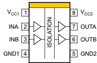
**Figure 4-1. ISO7220x D Package 8-Pin SOIC Top View**
