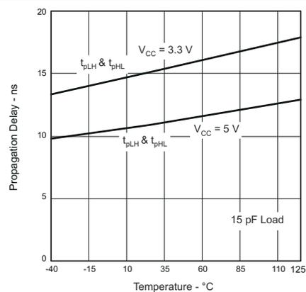
**Figure 5-7. Propagation Delay vs Free-Air Temperature, ISO722xM**
