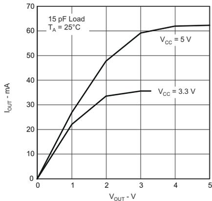
**Figure 5-12. Low-Level Output Current vs Low-Level Output Voltage**
