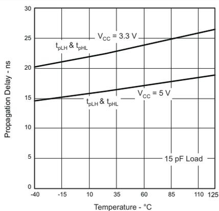
**Figure 5-6. Propagation Delay vs Free-Air Temperature, ISO722xC**
