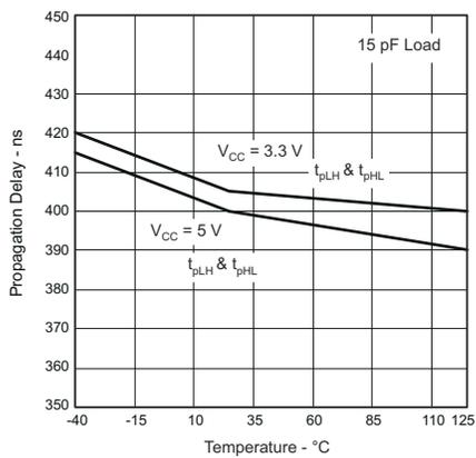
**Figure 5-4. Propagation Delay vs Free-Air Temperature, ISO722xA**
