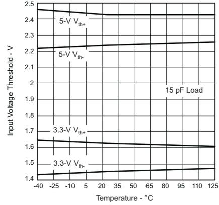
**Figure 5-9. ISO722xM Input Voltage High-to-Low vs Free-Air Temperature**
