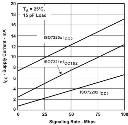
**Figure 5-2. 3.3-V<sub>RMS</sub> Supply Current vs Signaling Rate (Mbps)**
