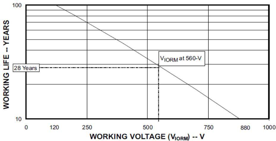
**Figure 8-4. Insulation Lifetime Projection**
