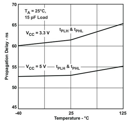
**Figure 5-5. Propagation Delay vs Free-Air Temperature, ISO722xB**
