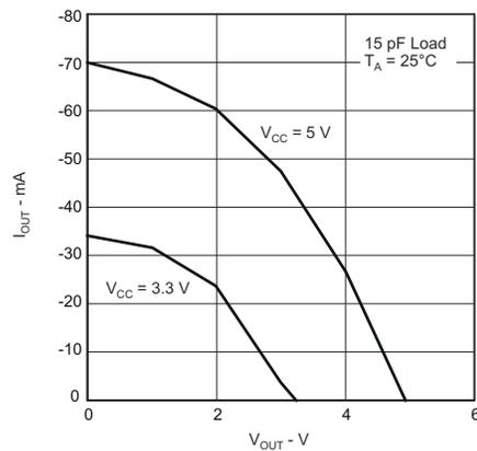
**Figure 5-11. High-Level Output Current vs High-Level Output Voltage**
