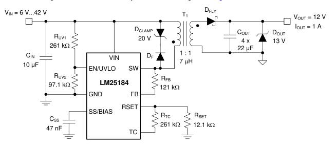
Figure 8-1. Schematic for Design 1 With  $V_{IN(nom)}$  = 24 V,  $V_{OUT}$  = 12 V,  $I_{OUT}$  = 1 A
