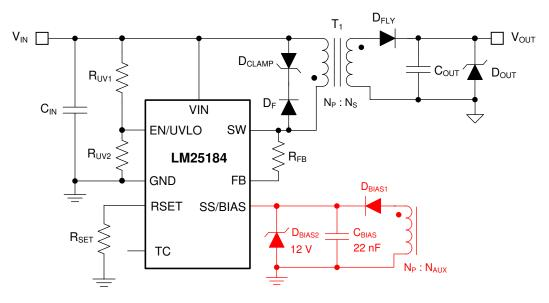
Figure 7-4. External Bias Supply Using Transformer Auxiliary Winding
