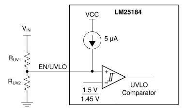
Figure 7-3. Programmable Input Voltage UVLO With Hysteresis
