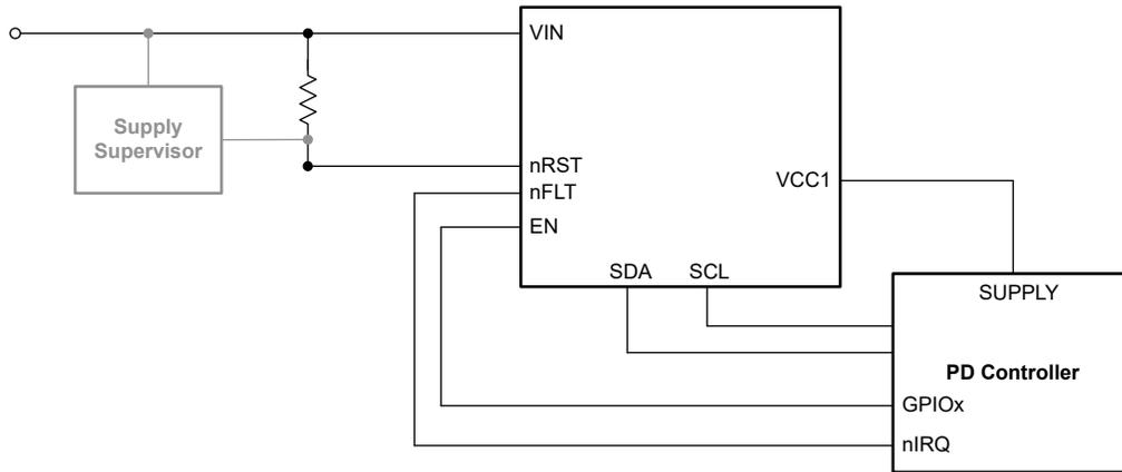
Figure 8-12. Simplified Schematic
