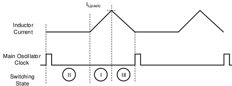
**Figure 8-5. Inductor Current in Continuous Buck-Boost Operation**
