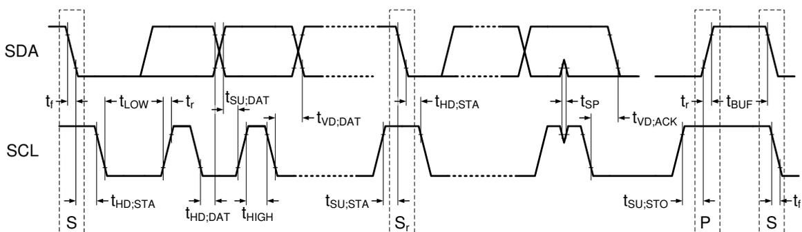
Figure 8-34. I<sup>2</sup>C Data Transmission Timing
