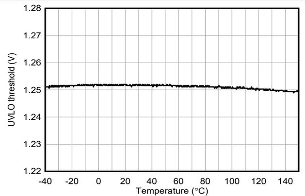
Figure 6-16. EN/UVLO Threshold versus Temperature
