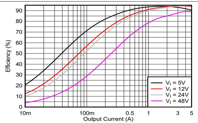
Figure 10-3. Efficiency Versus  $I_O$  (MODE = VCC2,  $V_O = 12V$ )
