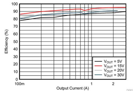
Efficiency vs. Output Current,  $V_i = 12V$ , PSM
