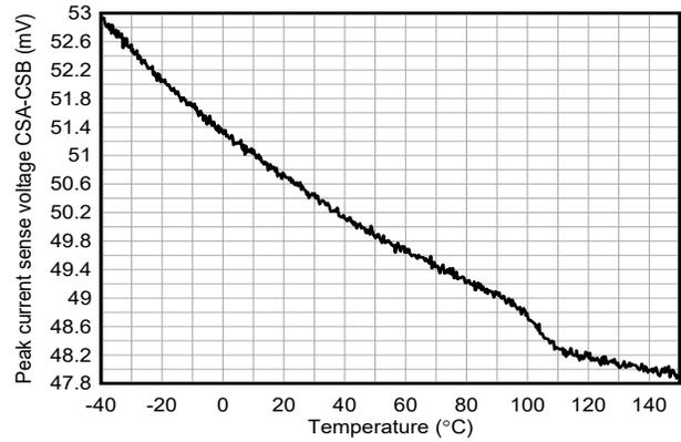
**Figure 6-28. Average Current Limit Threshold Voltage Versus Temperature
