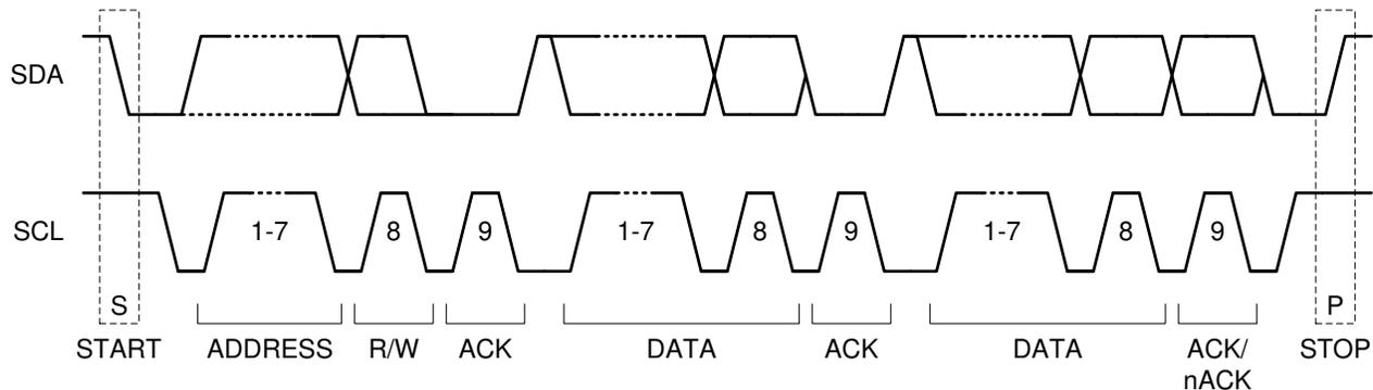
Figure 8-33. I<sup>2</sup>C START / STOP / ACKNOWLEDGE Protocol
