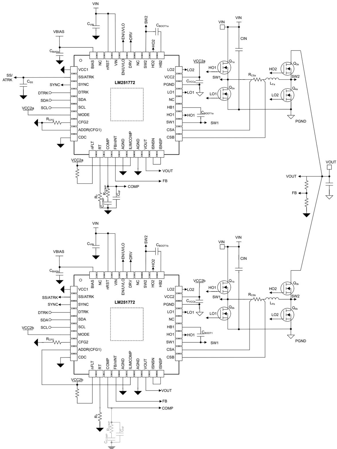
Figure 10-29. Simplified Schematic of a Two phase operation
