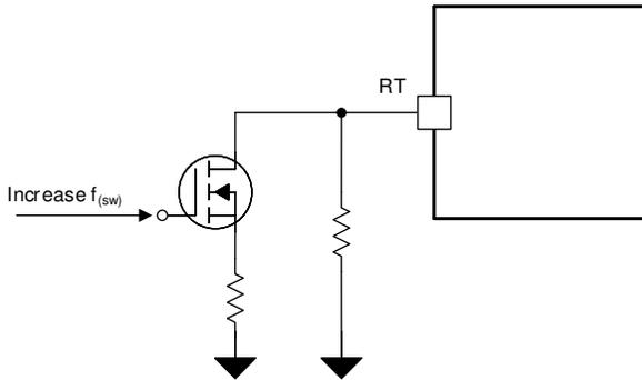
Figure 8-20. Frequency Hopping Example
