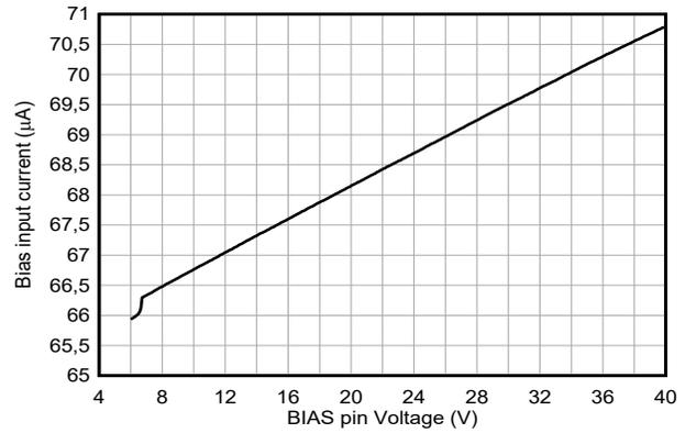
**Figure 6-8. Quiescent Current into BIAS versus BIAS pin voltage**
