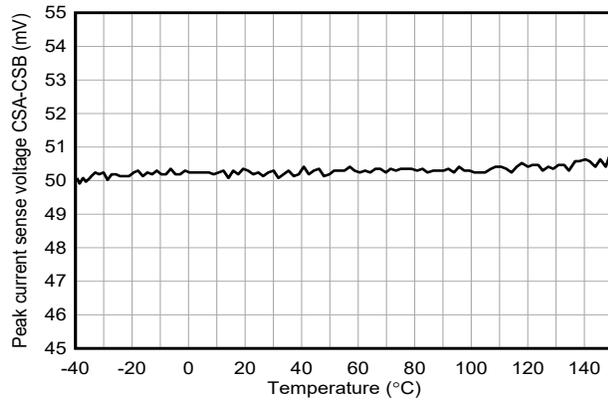
**Figure 6-25. Peak Current Limit Threshold Voltage Versus Temperature**
