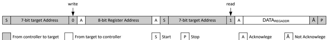
Figure 8-36. Single READ From a Defined Register Address
