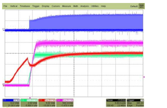
CH1: OUT, 10 V/div CH2: SS, 2 V/div CH3: VCC, 5 V/div CH4: VOUT, 5 V/div
