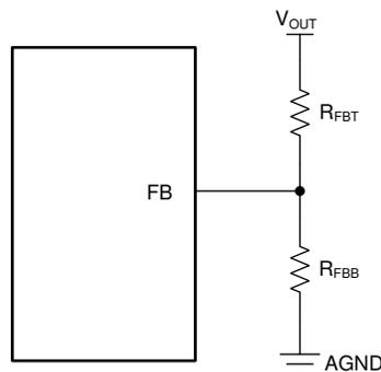
**Figure 9-11. Setting Output Voltage of Adjustable Versions**
