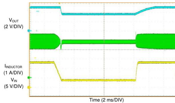
**Figure 9-10. Recovery From Dropout ( $V_{OUT} = 5\text{ V}$ ,  $I_{OUT} = 4\text{ A}$ ,  $V_{IN} = 13.5\text{ V}$  to  $4\text{ V}$  to  $13.5\text{ V}$ )**
