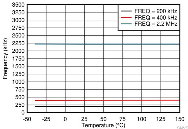
Figure 8-5. Switching Frequency Set by RT Resistor
