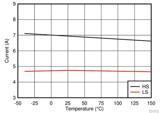
Figure 8-4. LM61440-Q1 High-side and Low-side Current Limits
