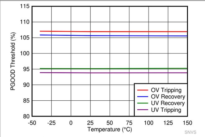
Figure 8-8. PGOOD Thresholds
