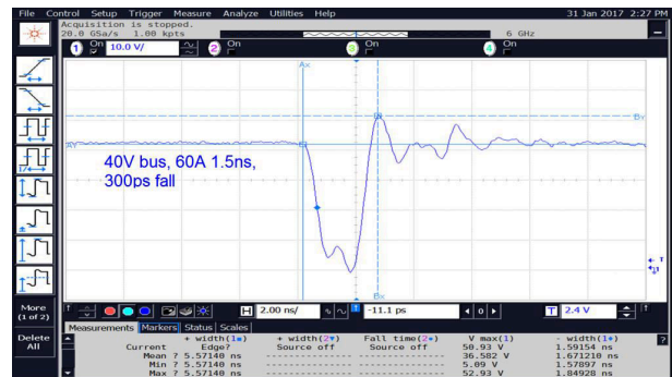
Figure 7-9. V_{DS} for 1.5ns Pulse with 40V of Bus Voltage
