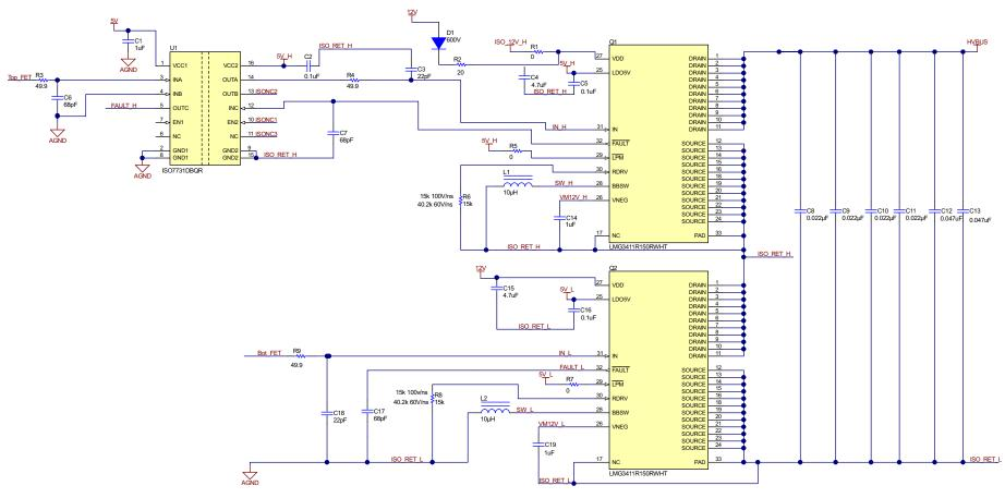
Figure 20. Typical Half-Bridge Application
