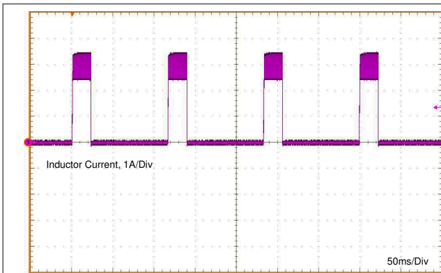
Figure 8-5. Inductor Current Burst in Short-Circuit Mode
