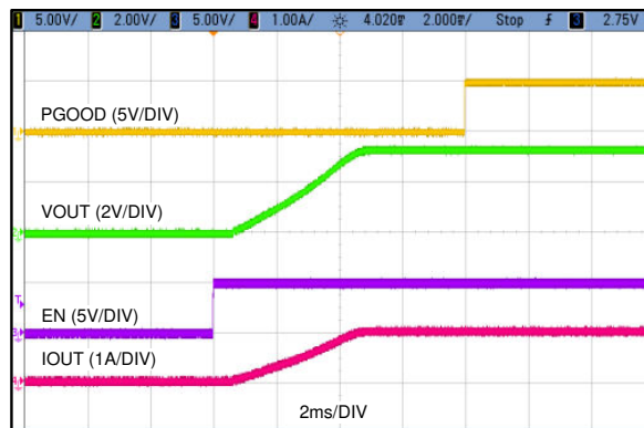
Figure 7-4. Typical Start-up Behavior V_{IN} = 24\text{ V} , V_{OUT} = 5\text{ V} , I_{OUT} = 1\text{ A}
