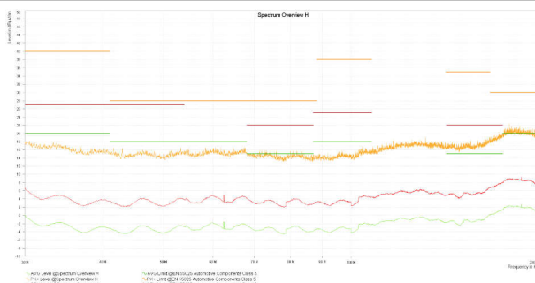
Figure 8-26. Radiated EMI Monopole versus CISPR25 Limits, LMR60440QEV
