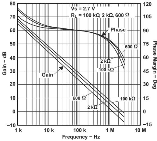
Figure 6-1. LMV321 Frequency Response vs Resistive Load
