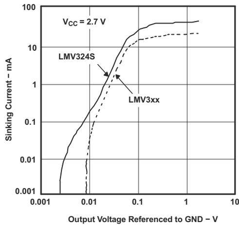
Figure 6-15. Sinking Current vs Output Voltage
