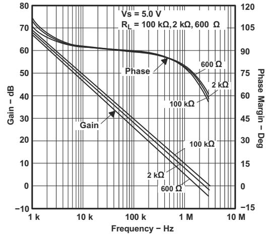
Figure 6-2. LMV321 Frequency Response vs Resistive Load
