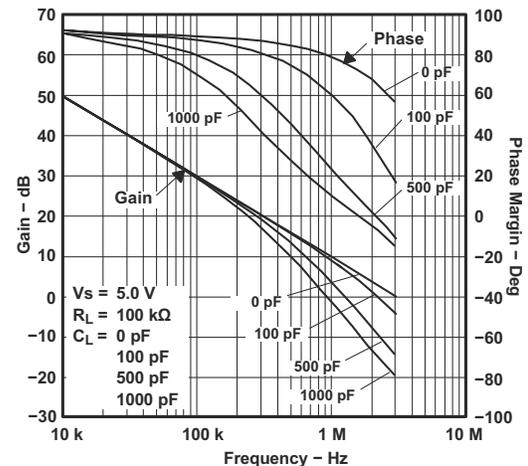
Figure 6-4. LMV321 Frequency Response vs Capacitive Load
