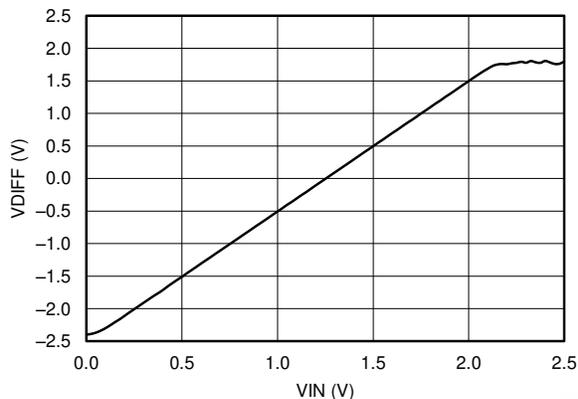
**Figure 8-2. Differential Output Voltage vs Input Voltage**
