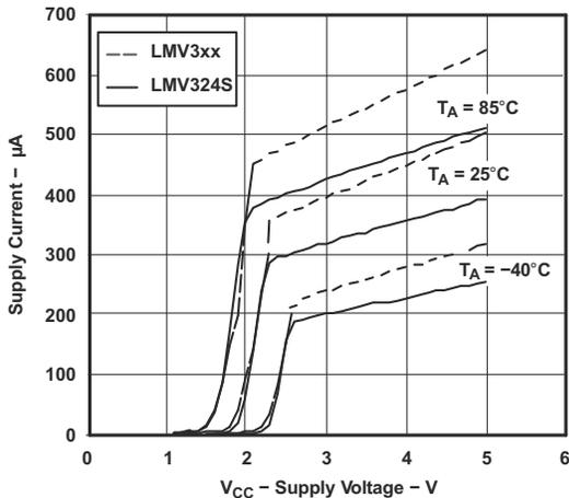
Figure 6-11. Supply Current vs Supply Voltage: Quad Amplifier
