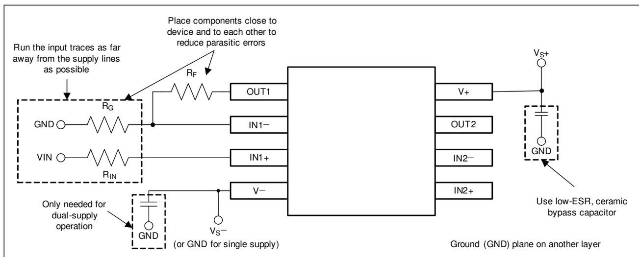
**Figure 8-6. Operational Amplifier Board Layout for Noninverting Configuration**
