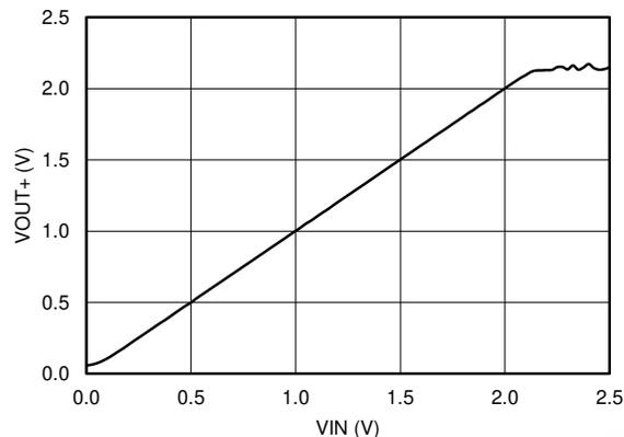
**Figure 8-3. Positive Output Voltage Node vs Input Voltage**
