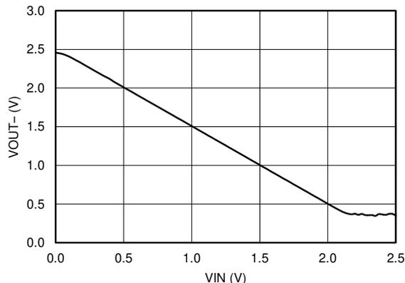
**Figure 8-4. Positive Output Voltage Node vs Input Voltage**
