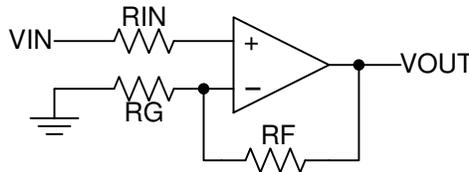
**Figure 8-5. Operational Amplifier Schematic for Noninverting Configuration**
