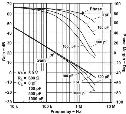
Figure 6-3. LMV321 Frequency Response vs Capacitive Load
