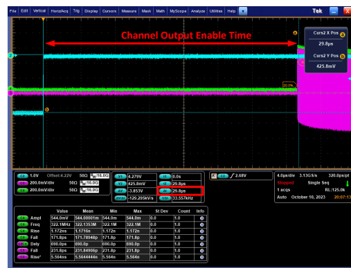
Figure 5-19. Channel Enable Setting Time
