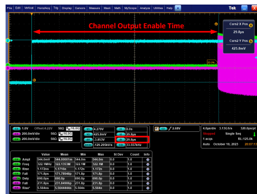
Figure 5-19. Channel Enable Setting Time
