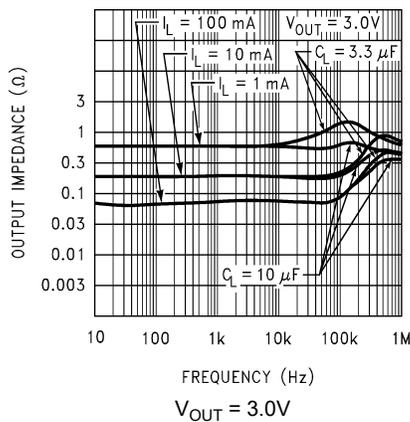
**Figure 5-39. Output Impedance vs Frequency (Legacy Chip)**
