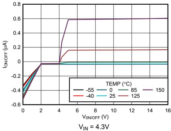
Figure 5-55.  $\text{ON}/\overline{\text{OFF}}$  Pin Current vs  $V_{\text{ON}/\overline{\text{OFF}}}$  (New Chip)
