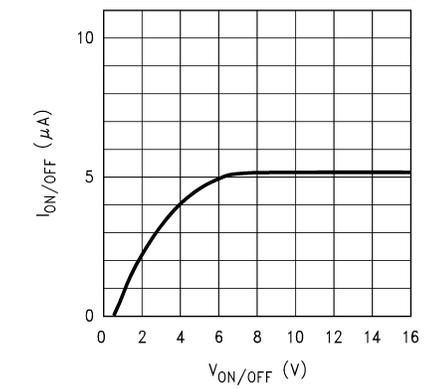
**Figure 5-54. ON/OFF Pin Current vs  $V_{ON/OFF}$  (Legacy Chip)**
