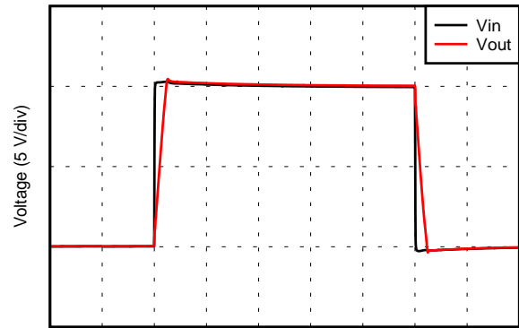
Figure 34. Small-Signal Step Response (Noninverting)
