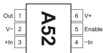
Figure 4-1. OPA300, SOT-23 Package, 6-pin (Top View)
