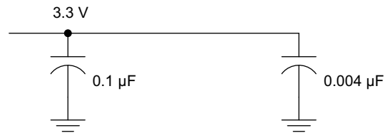
Figure 9-2. Recommended M-LVDS Bypass Capacitor Layout
