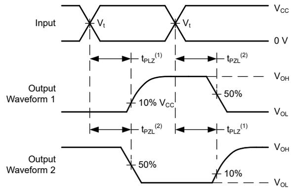
(1)  $t_{\text{PLZ}}$  is the same as  $t_{\text{dis}}$ .
