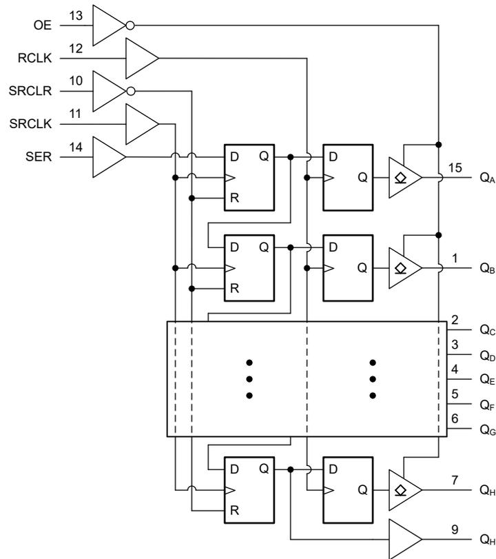
Figure 7-1. Logic Diagram (Positive Logic) for SN74ACT596
