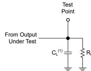
(1)  $C_L$  includes probe and test-fixture capacitance.
