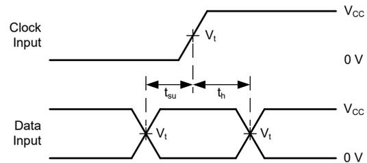
**Figure 6-4. Voltage Waveforms, Setup and Hold Times**
