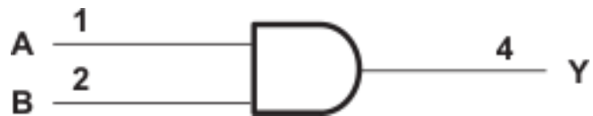
Logic Diagram (Positive Logic)
