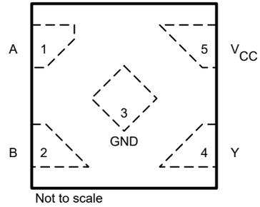
**Figure 4-2. DTX Package, 5-Pin X2SON (Top View)**
