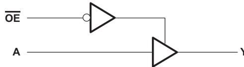
**Simplified Logic Diagram (Positive Logic)**
