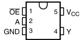
Figure 5-1. SN74AHC1G125-Q1 DBV Package, 5-Pin SOT-23; DCK Package, 5-Pin SC-70 (Top View)
