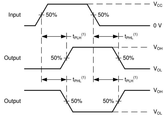
(1) The greater between t<sub>PLH</sub> and t<sub>PHL</sub> is the same as t<sub>pd</sub>.
