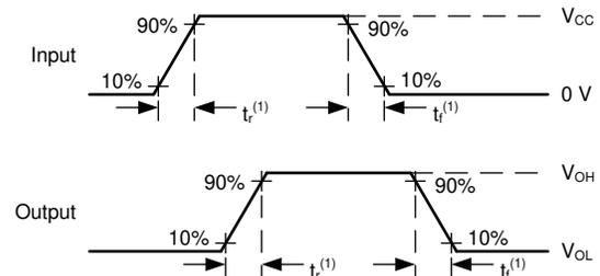
(1) The greater between t<sub>r</sub> and t<sub>f</sub> is the same as t<sub>t</sub>.
