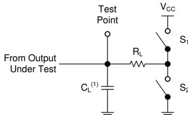
(1) C<sub>L</sub> includes probe and test-fixture capacitance.
