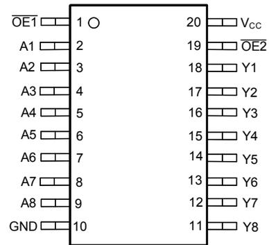
**Figure 4-2. SN74AHC9541-Q1 PW, DGS Package (Top View)**
