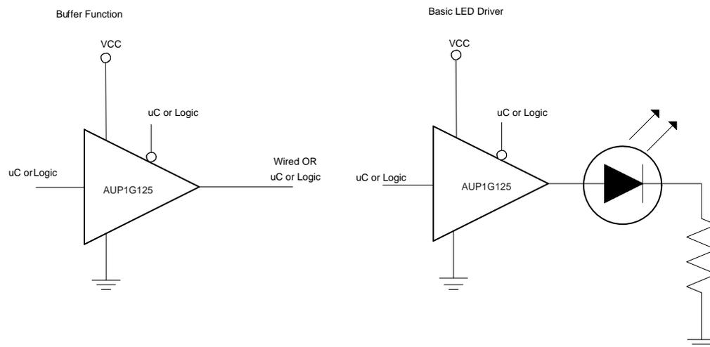
**Figure 5. Application Schematic**
