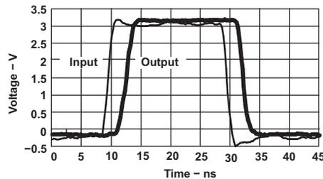
Figure 6. Switching Characteristics at 25 MHz
