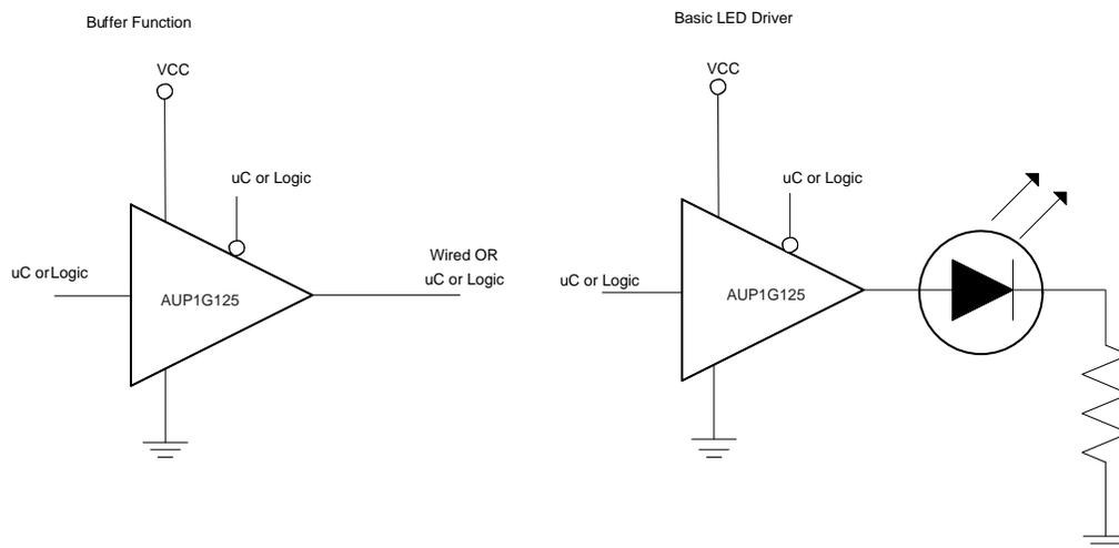
**Figure 5. Application Schematic**
