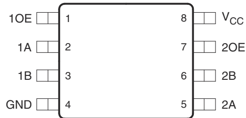
Figure 5-2. DCU Package 8-Pin VSSOP Top View
