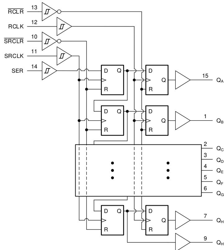
Figure 8-1. Logic Diagram (Positive Logic) for SN74HCS594-Q1
