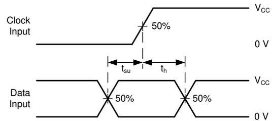
Figure 7-4. Voltage Waveforms, Setup and Hold Times
