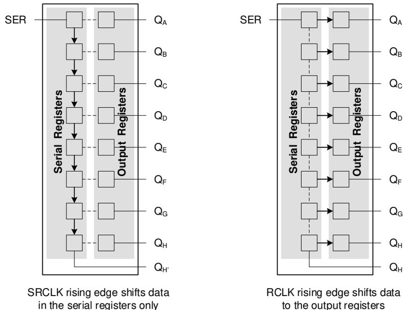
**Figure 9-2. Simplified functional diagram showing clock operation**
