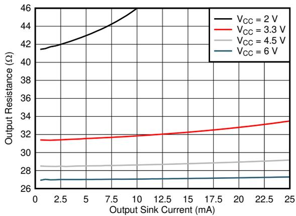
Figure 6-2. Output driver resistance in LOW state.
