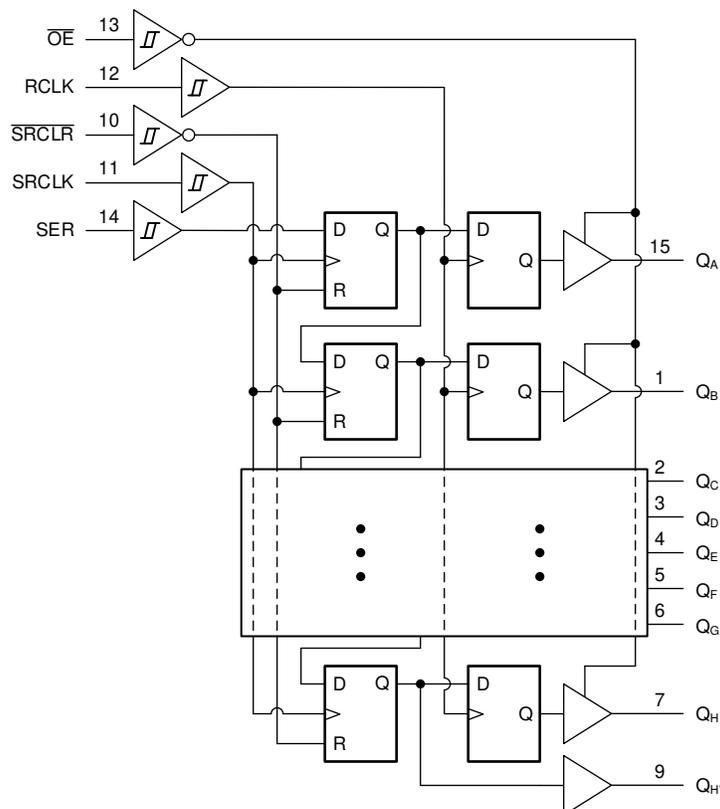
Figure 8-1. Logic Diagram (Positive Logic) for the SN74HCS595
