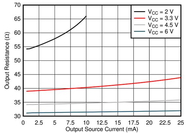
Figure 6-3. Output driver resistance in HIGH state.
