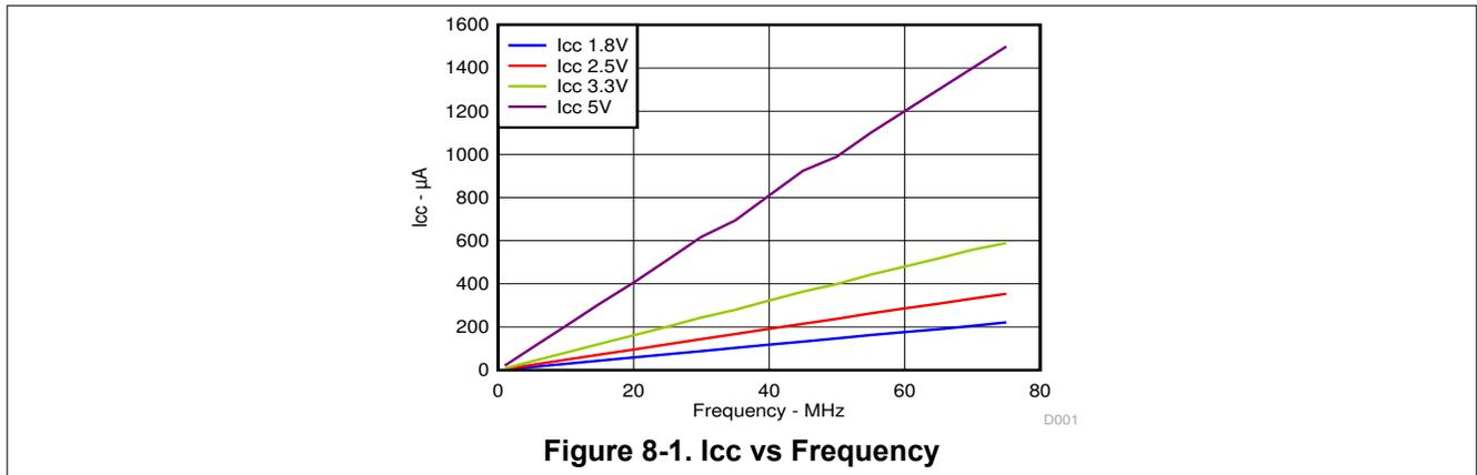
Figure 8-1. Icc vs Frequency
