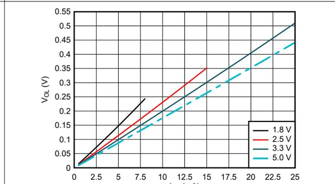
Figure 5-4. Output Voltage vs Current in LOW State
