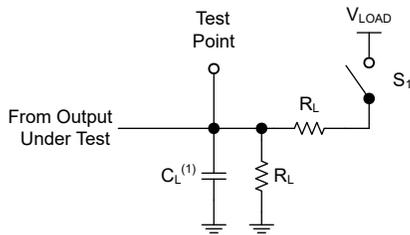
(1) C<sub>L</sub> includes probe and test-fixture capacitance.
