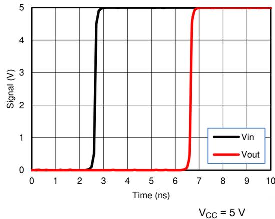
**Figure 8-2. Simulated Input-to-Output Voltage Response Showing Propagation Delay**
