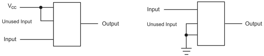
Figure 8-3. Layout Diagrams
