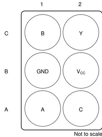
**Figure 4-2. YZP Package 6-Pin DSBGA (Bottom View)**
