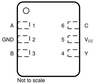
**Figure 4-3. DRY Package 6-Pin SON (Top View)**
