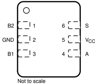
**Figure 4-5. DSF Package, 6-Pin SON (Top View)**
