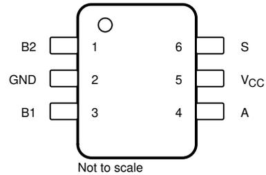
**Figure 4-4. DRL Package, 6-Pin SOT (Top View)**
