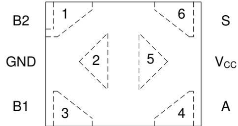
**Figure 4-6. DTB Package, 6-Pin X2SON (Top View)**
