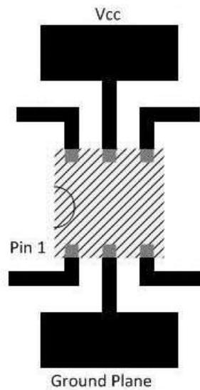
Figure 10-1. Recommended Layout Example
