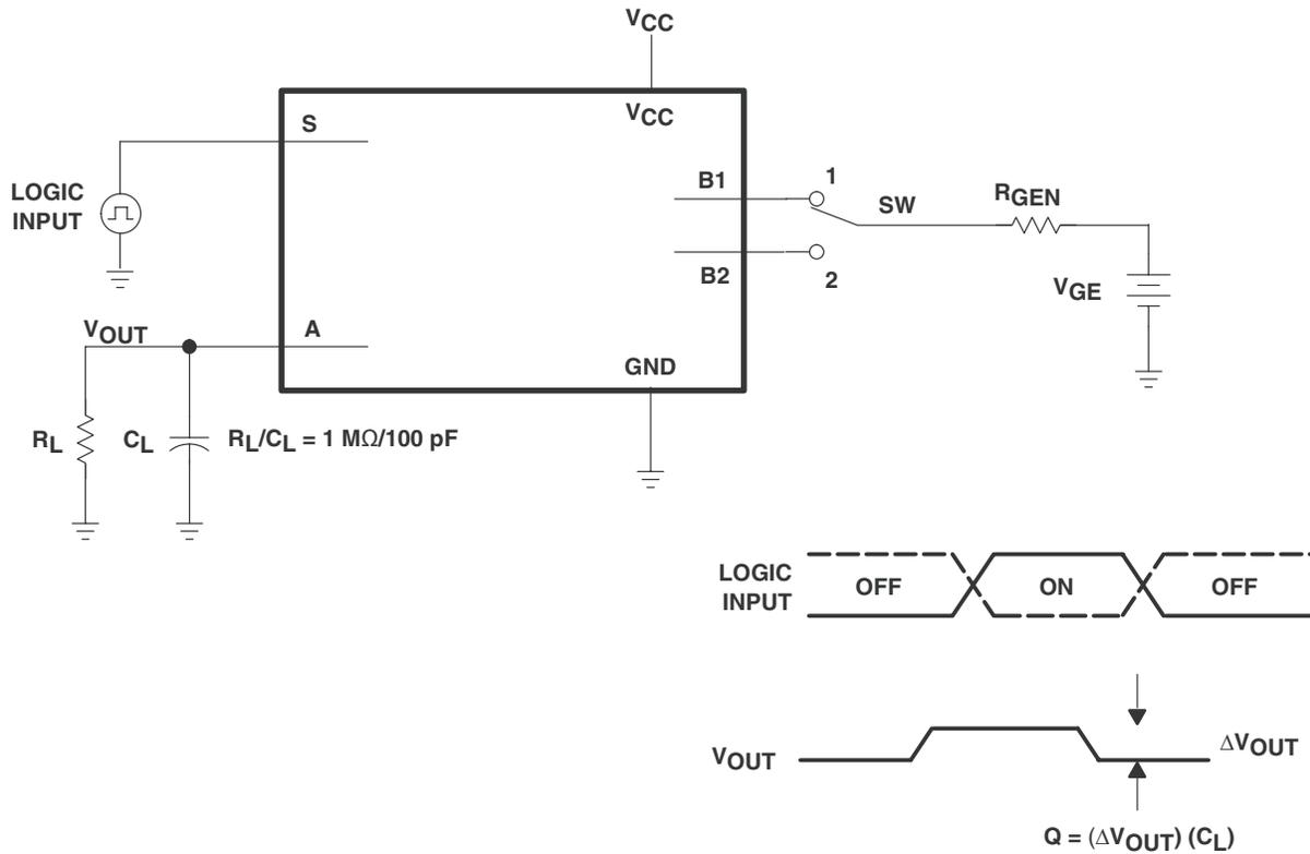
Figure 6-8. Charge-Injection Test
