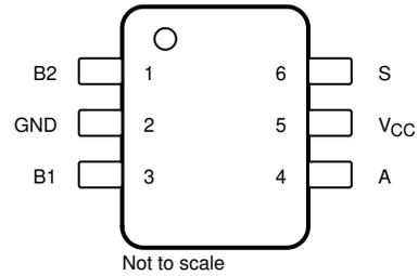
**Figure 4-2. DCK Package, 6-Pin SC70 (Top View)**
