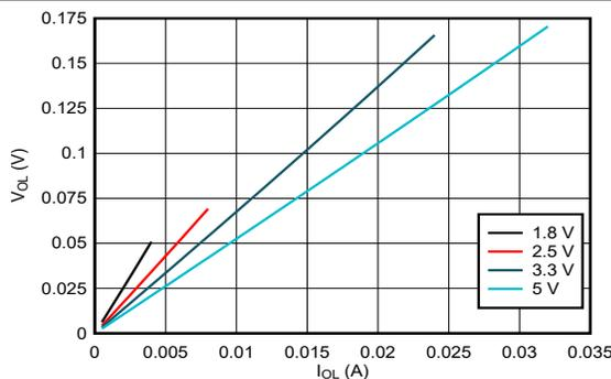
Figure 5-3. Output Voltage vs Current in LOW State
