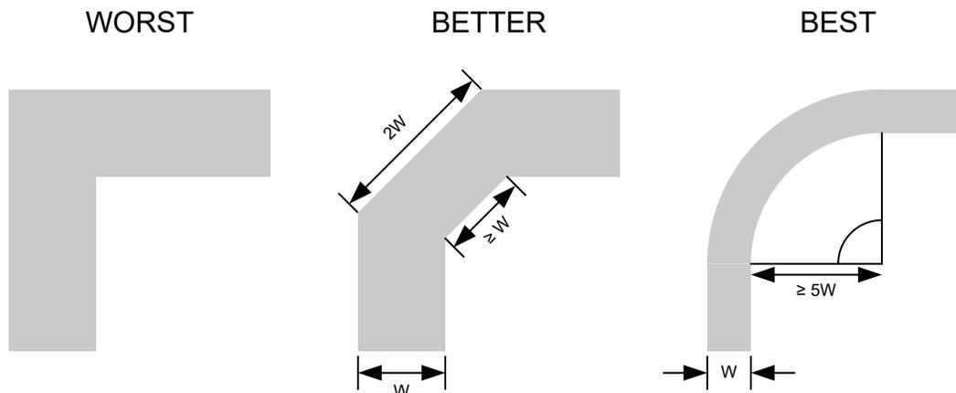
Figure 8-3. Example Trace Corners for Improved Signal Integrity
