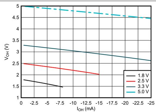
Figure 5-2. Output Voltage vs Current in HIGH State
