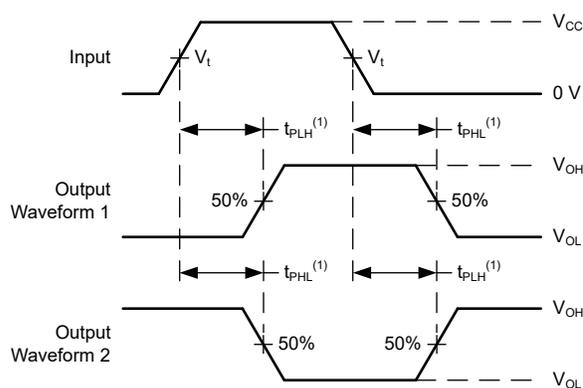
(1) The greater between t<sub>pLH</sub> and t<sub>pHL</sub> is the same as t<sub>pd</sub>.
