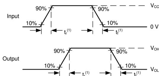
(1) The greater between t<sub>r</sub> and t<sub>f</sub> is the same as t<sub>t</sub>.
