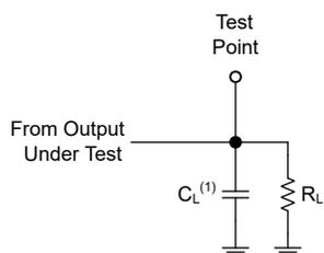
(1) C<sub>L</sub> includes probe and test-fixture capacitance.
