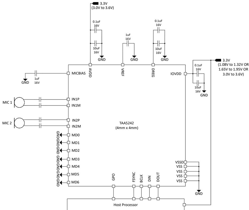
Figure 9-1. Stereo MEMS Microphone Block Diagram
