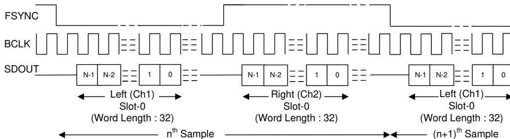
Figure 8-4. I<sup>2</sup>S Mode Protocol Timing (MD0 shorted to ground) in Target Mode
