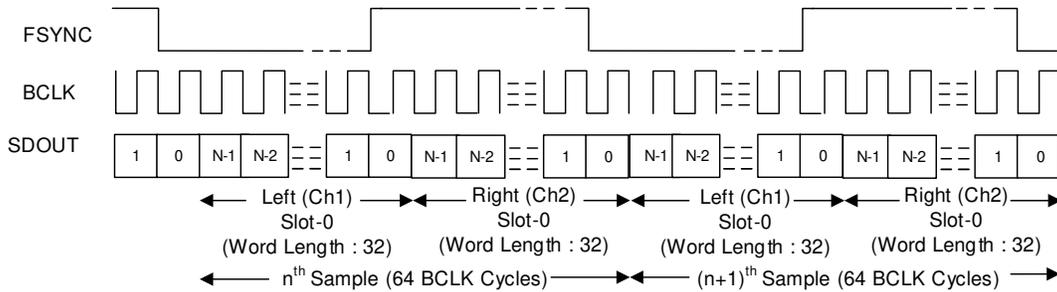
**Figure 8-5. I<sup>2</sup>S Protocol Timing (MD0 shorted to AVDD) In Controller Mode**
