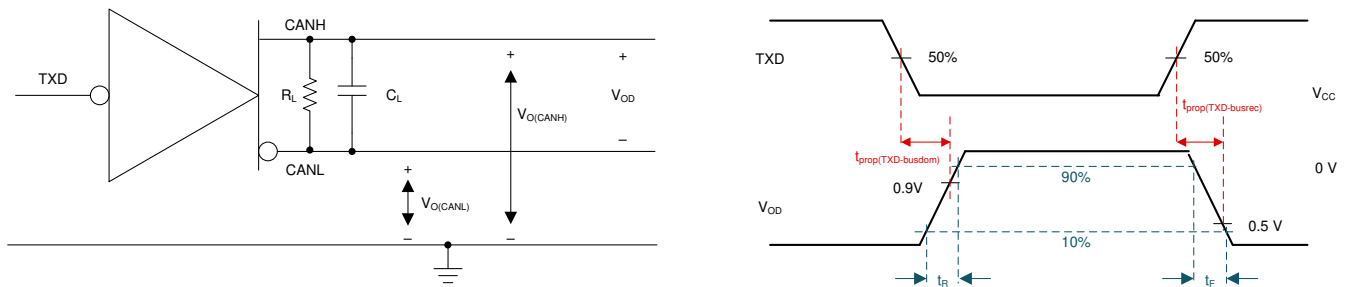
Figure 7-2. Driver Test Circuit and Measurement
