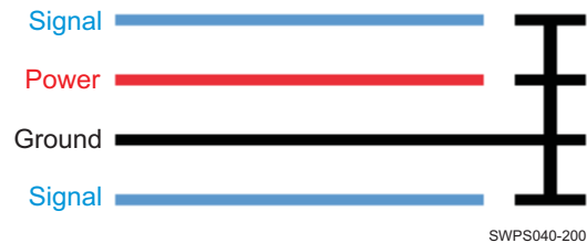
Figure 7-19. Guard Ring Routing
