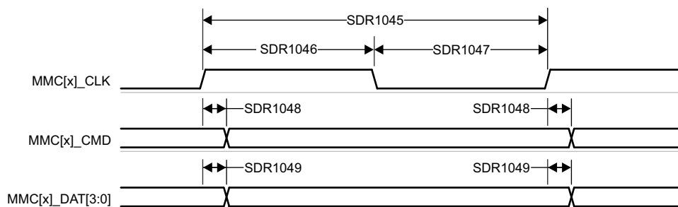
Figure 7-95. MMC1/2 – UHS-I SDR104 – Transmit Mode
