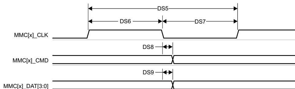
Figure 7-86. MMC1/2 – Default Speed – Transmit Mode
